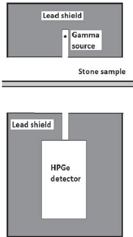
**Figure 2.** Schematic diagram of the Geant4 set-up.
