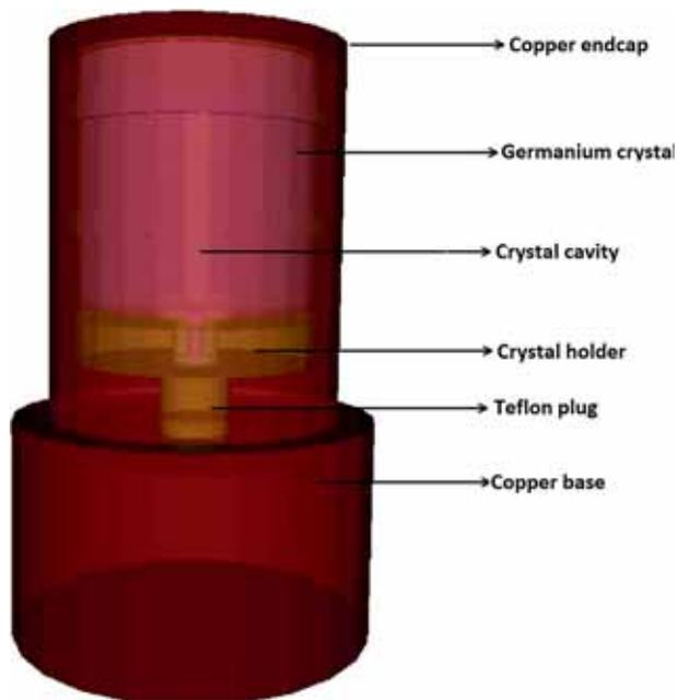
**Figure 1.** Geant4 model of the HPGe detector used for determining mass attenuation coefficient.
