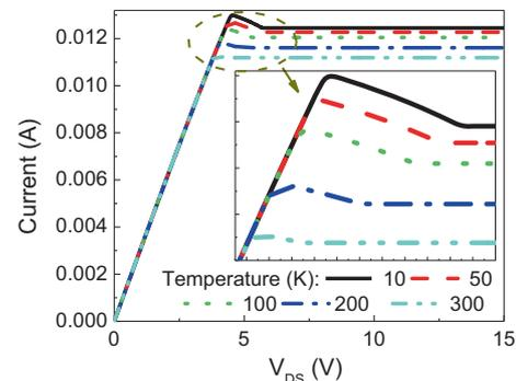
**Figure 5.** The source–drain current as a function of the source–drain voltage at the largest electron drift velocity of  $5 \times 10^5$  m/s for different lattice temperatures.
