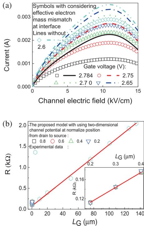
**Figure 10.** (a) The source–drain current as a function of source–drain voltage and (b) the channel resistance as a function of the gate length of GaN HEMT.
