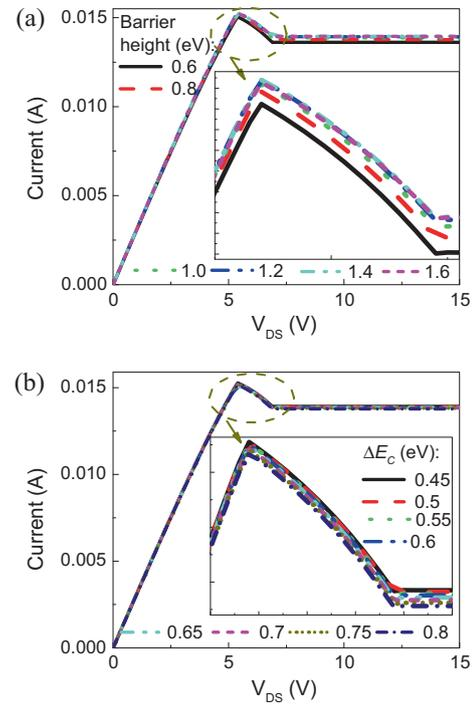
**Figure 8.** The source–drain current as a function of the source–drain voltage at the largest electron drift velocity of  $7 \times 10^5$  m/s for (a) different Schottky barrier height and (b) conduction band offset between  $\text{Al}_{0.3}\text{Ga}_{0.7}\text{N}$  and GaN.
