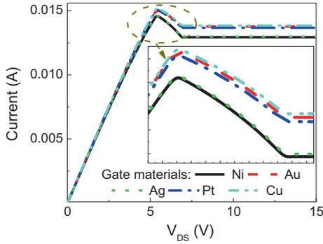
**Figure 6.** The source–drain current as a function of the source–drain voltage at the largest electron drift velocity of  $7 \times 10^5$  m/s for different gate metals.
