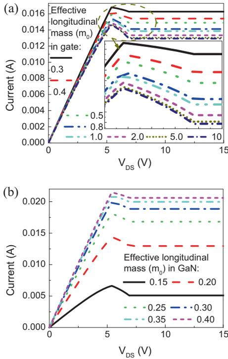
**Figure 7.** The source–drain current as a function of the source–drain voltage at the largest electron drift velocity of  $7 \times 10^5$  m/s for different effective longitudinal electron mass of (a) the gate and (b) GaN.
