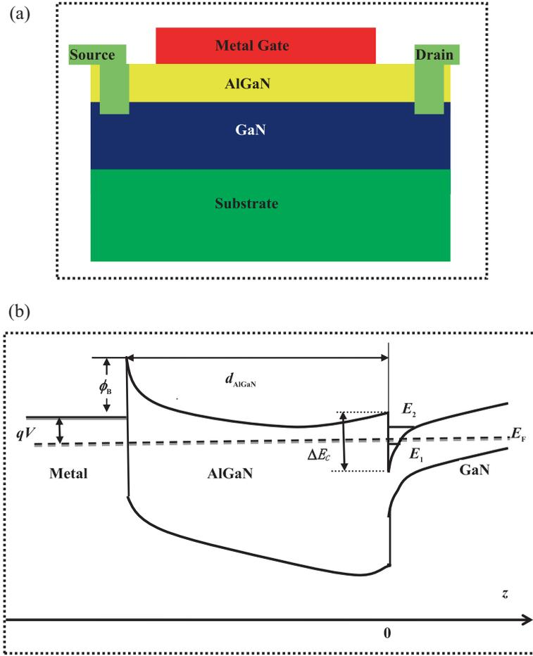
**Figure 1.** (a) Schematic cross-section and (b) the band diagram of the AlGaIn/GaN HEMTs conventional structure.
