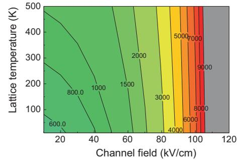
**Figure 3.** Contour of the electron temperature in GaN HEMTs between the channel electric field and the lattice temperature.
