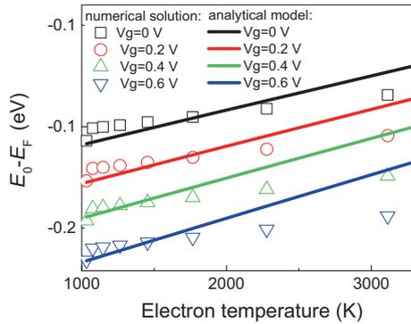
**Figure 2.** The comparison of the first quantised energy levels as a function of electron temperature calculated by the proposed analytical model and the numerical calculations.
