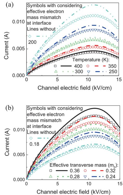
**Figure 9.** The source–drain current as a function of source–drain voltage when the gate material is Au for (a) different lattice temperatures and (b) different effective transverse electron mass of GaN.
