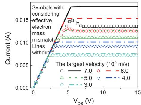
**Figure 4.** The source–drain current as a function of source–drain voltage with and without considering the quantum coupling.
