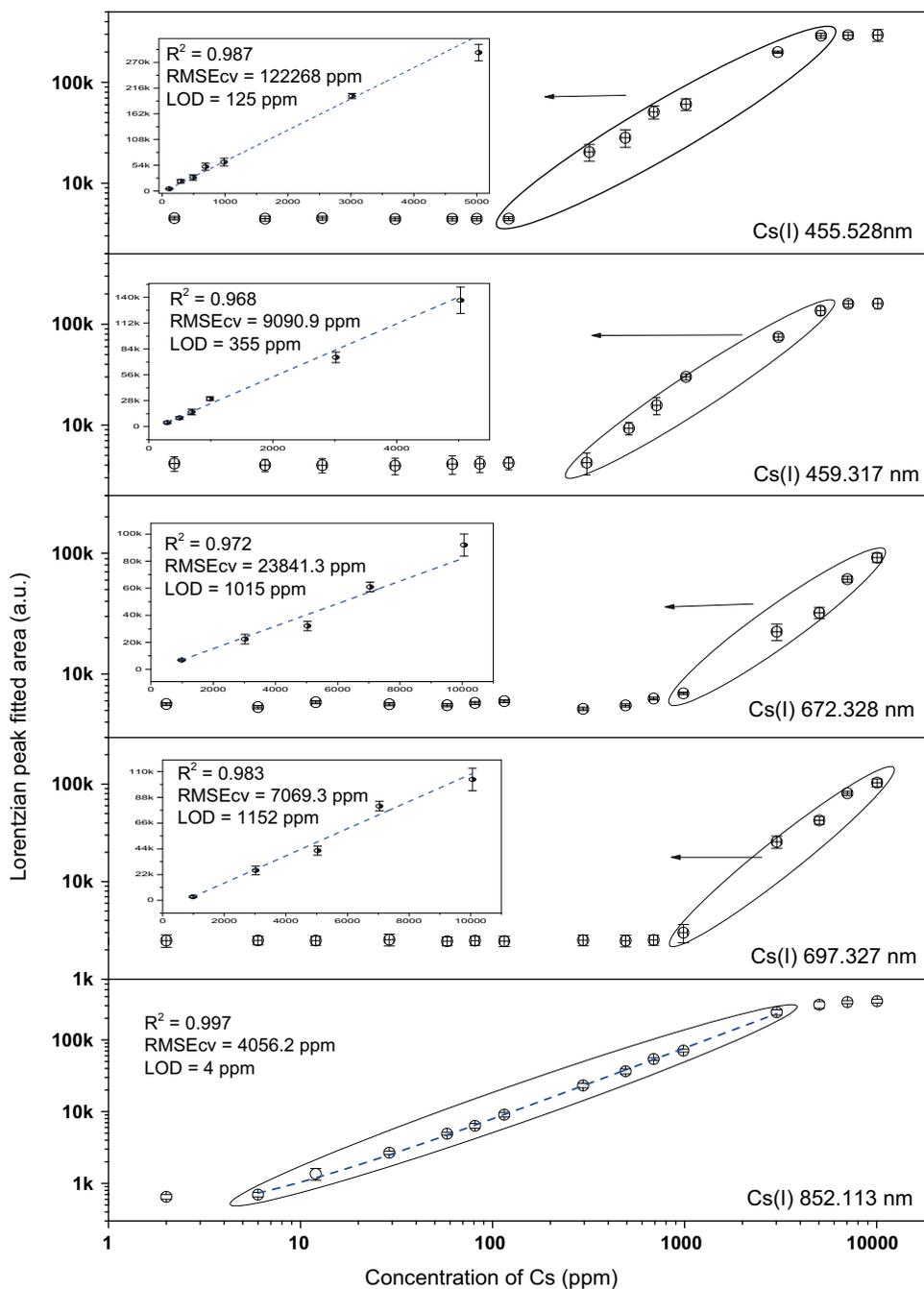
**Figure 3.** Dynamic range and the constructed calibration curves in the respective dynamic range for the Cs(I) (455.53 nm), Cs(I) (459.33 nm), Cs(I) (672.33 nm), Cs(I) (697.33 nm) and Cs(I) (852.11 nm).
