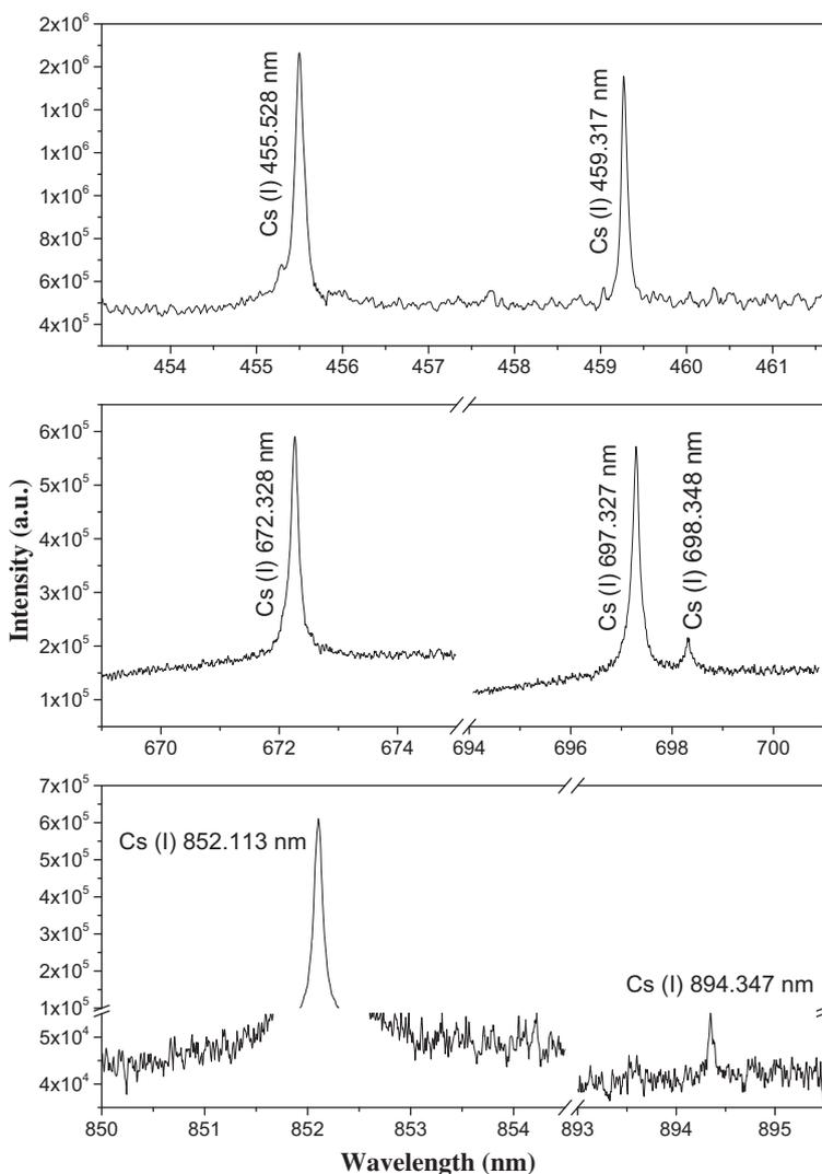
**Figure 1.** Accumulation of 60 single-shot LIBS spectra of Cs solution on a graphite planchet at a laser energy of 50 mJ and acquisition delay of 2  $\mu s$ .
