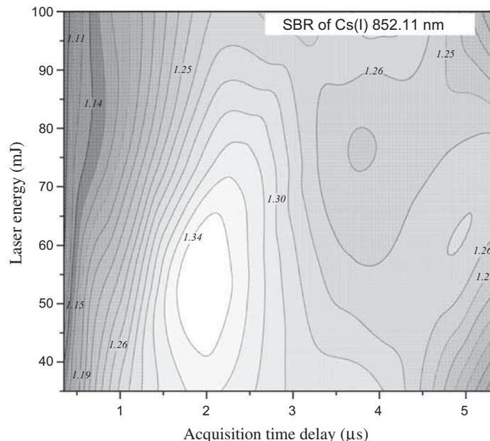
**Figure 2.** Contour diagrams of Cs(I) (852.11 nm) emission line showing the effects of  $t_d$  and  $E_L$  on the SBR.
