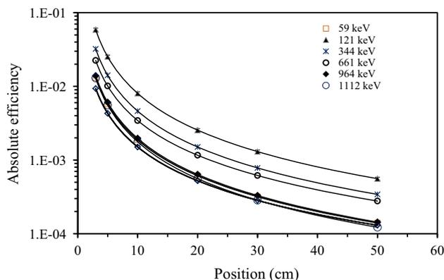
**Figure 3.** Variation of measured efficiencies with source–detector distances for the particular  $\gamma$ -ray energy.
