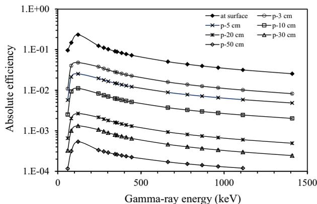
**Figure 2.** Efficiency vs. energy curves at various source–detector distances.
