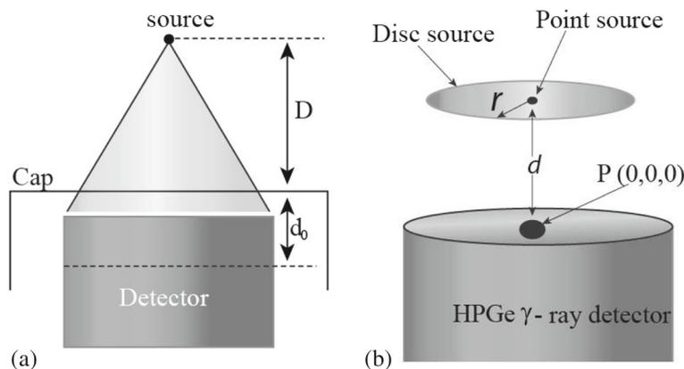
**Figure 1.** Geometry of HPGe  $\gamma$ -ray detector. (a) Geometric basis of the correction for source-to-detector distance and (b) geometry of a disc source of infinitesimal thickness and an equivalent point source on the detector axis.
