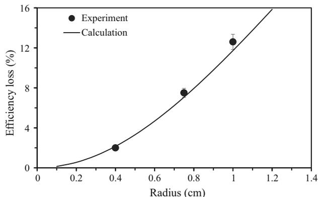
**Figure 4.** Variation of loss of efficiency in extended disc source with that of the point source at the detector surface.
