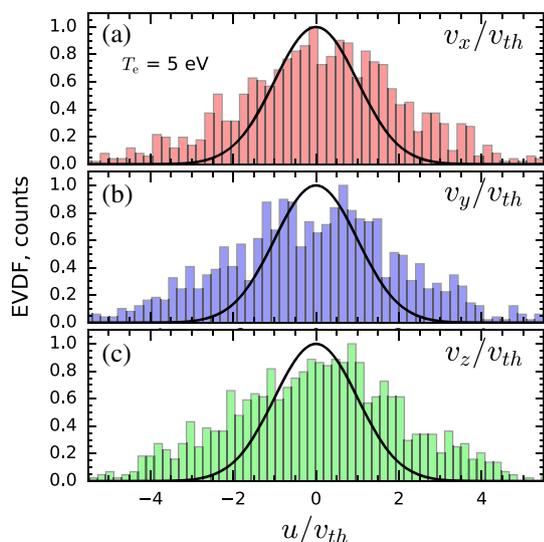
**Figure 4.** Distribution of velocity components ( $u = v_x, v_y, v_z$ ) of electrons in units of  $v_{th}$  corresponding to the parameters of figure 2b at an intensity of  $5 \times 10^{14} \text{ W cm}^{-2}$  just after the end of the simulation. Solid line is the expected Maxwellian with  $T_e = 5 \text{ eV}$ .
