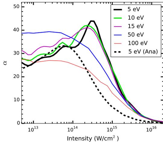
**Figure 3.** Fractional absorption vs. peak laser intensity for  $s$ -polarised light interacting with an under-dense plasma as in figure 2 for  $T_e = 5, 10, 15, 50, 100$  eV (numerical, solid line) and  $T_e = 5$  eV (analytical, dashed line, using eq. (21)).
