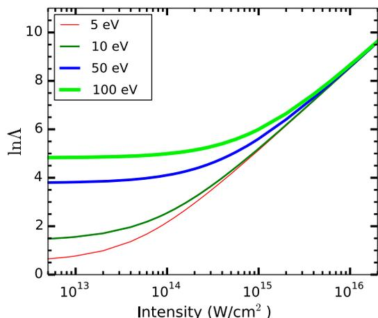
**Figure 1.**  $\ln \Lambda$  vs. laser intensity for  $T_e = 5, 10, 50$  and  $100$  eV with total velocity  $v = (v_{th}^2 + v_0^2/2)^{1/2}$  and charge density  $\rho = 0.136\rho_c$ .
