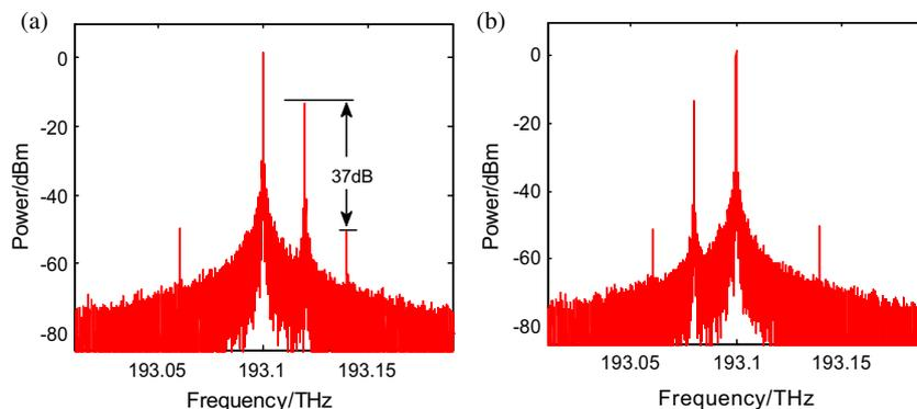
**Figure 5.** Optical spectra from (a) port 1 and (b) port 2 of the dual-output DPMZM.
