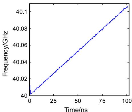
**Figure 8.** Instantaneous frequency of the generated pulse.
