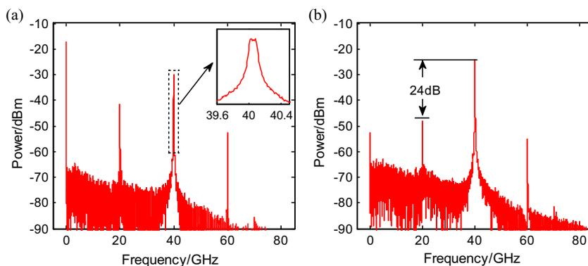
**Figure 6.** Electrical spectra for the signals generated by (a) single-end and (b) balanced detection.
