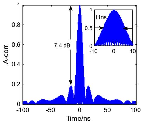
**Figure 9.** Autocorrelation function of the generated pulse.
