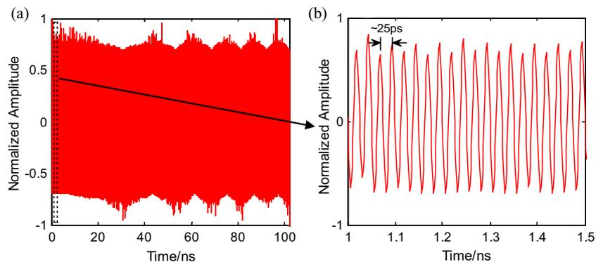
**Figure 7.** Generated pulse waveforms (a) with full time duration and (b) zoom-in with a time span of 1 to 1.5 ns.
