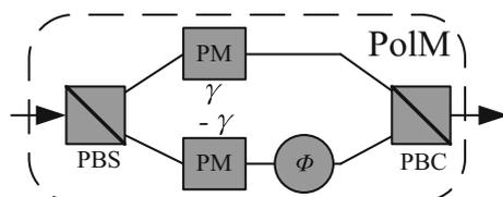
Figure 4. Polarisation modulator.
