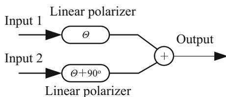
Figure 3. Polarisation beam combiner.
