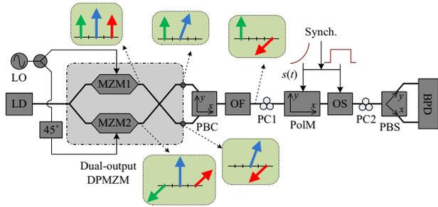
**Figure 1.** Schematic of the proposed chirped mm-wave pulse generation. LO, local oscillator; LD, laser diode; DPMZM, dual-parallel Mach–Zehnder modulator; PBC, polarisation beam combiner; OF, optical filter; PC, polarisation controller; PolM, polarisation modulator; OS, optical switch; PBS, polarisation beam splitter; BPD, balanced photodetector.
