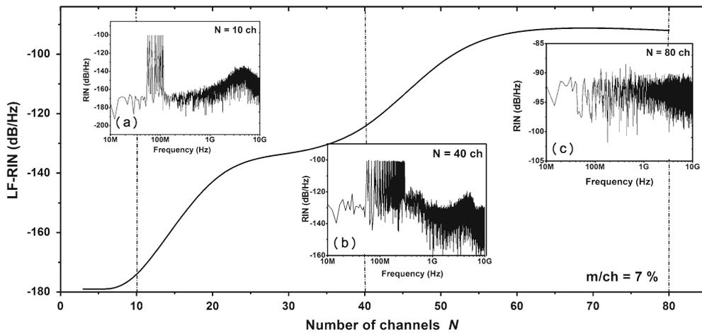
**Figure 4.** Variation of laser LF-RIN with the number of channels  $N$  when  $m/ch = 7\%$ . The insets are spectra of RIN when  $N = 10, 40,$  and  $80$ .
