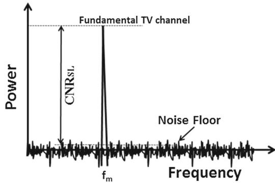
**Figure 1.** Scheme illustrating calculation of CNR of the laser signal.
