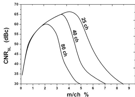
**Figure 5.** Variation of  $CNR_{SL}$  with  $m/ch$  under 25, 40, and 80 channels. The three peaks are the optimum values of  $CNR_{SL}$ .
