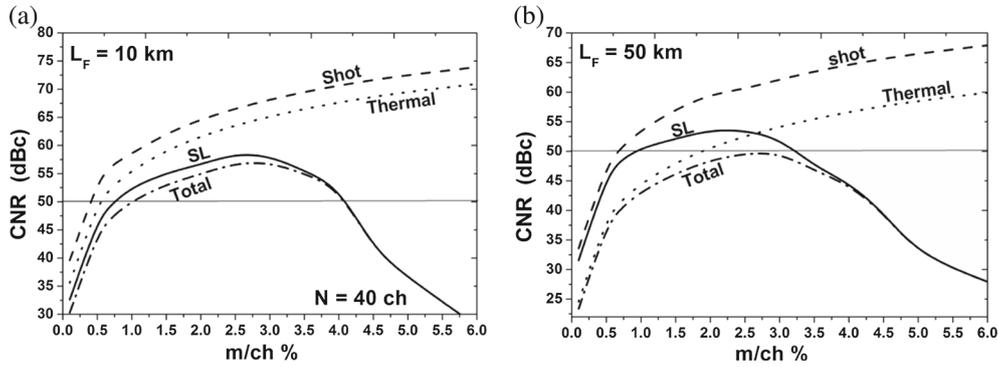
**Figure 6.** CNR due to laser RIN (solid line), receiver shot noise (dashed line), and thermal noise (dotted line) as well as total link CNR (dash–dotted line) as functions of  $m/ch$  when (a)  $L_F = 10$  km and (b)  $L_F = 50$  km while loading 40 channels. The straight solid line represents the threshold acceptable levels of total link CNR.
