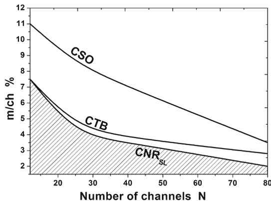
**Figure 7.** Optimum value of  $m/ch$  as a function of the number of channels that correspond to acceptable levels of CSO, CTB, and  $CNR_{SL}$  (corresponding to the shadow area).
