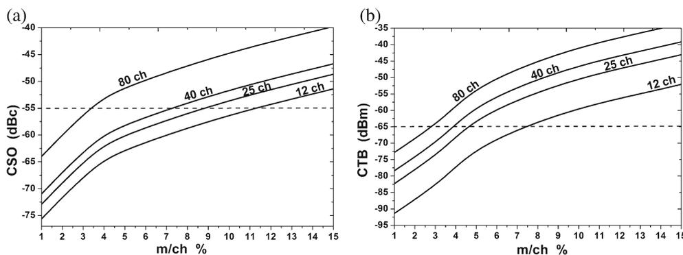
**Figure 2.** Variation of (a) CSO and (b) CTB distortions with modulation index per channel  $m/ch$  under 12, 25, 40, and 80 channels at ch. 12. The dashed lines represent the threshold acceptable levels.
