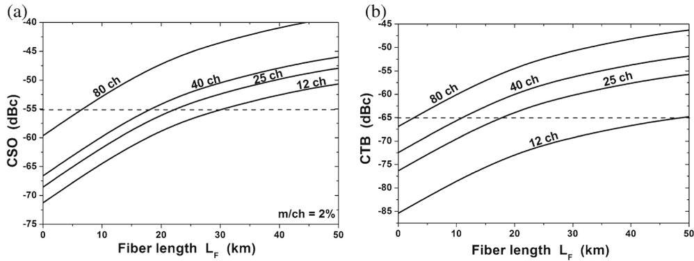
**Figure 3.** Variation of (a) CSO and (b) CTB with  $L_F$  under 12, 25, 40, and 80 channels when  $m/ch = 2\%$  at ch. 12. The dashed lines represent the threshold acceptable levels.
