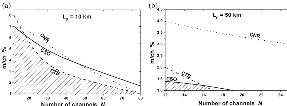
**Figure 8.** Optimum value of  $m/ch$  as a function of  $N$  that correspond to acceptable levels of CSO, CTB, and CNR for CATV fibre link when (a)  $L_F = 10$  km and (b)  $L_F = 50$  km. The shadow areas correspond to the optimum ranges of  $m/ch$  and  $N$ .
