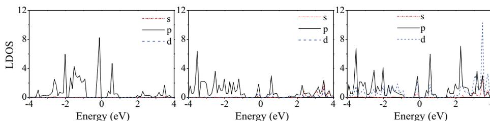
**Figure 3.** LDOS onto the (left) O atom, (centre) C atom and (right) Si atom of 7-ASiCNR-O.
