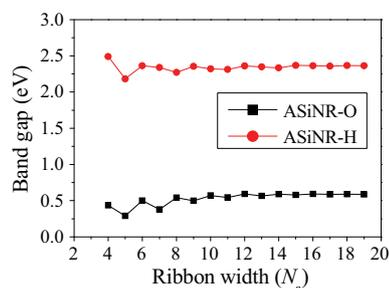
**Figure 6.** Variation of the energy band gap as a function of the ribbon width  $N_a$  for ASiCNRs-O and -H.
