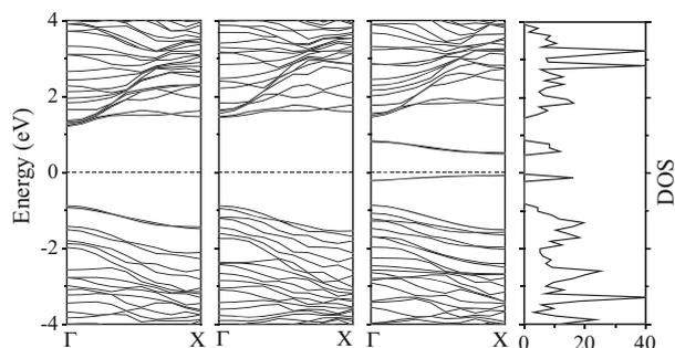
**Figure 4.** From the left to the right panels, band structures of 13-ASiCNRs-F, -H and -O as well as the total DOS of 13-ASiCNR-O are shown. The Fermi level set to zero is indicated by black dashed lines.
