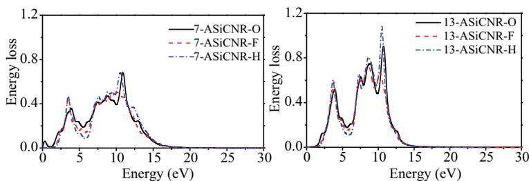
**Figure 10.** The energy loss coefficient of O-, F- and H-terminated 7-ASiCNRs and 13-ASiCNRs. The black solid, red dashed and blue dashed dot lines indicate the energy-loss coefficients of O-, F- and H-terminated ASiCNRs, respectively.
