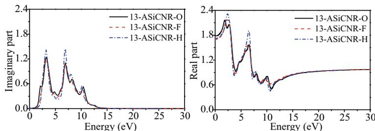
**Figure 8.** The theoretically calculated dielectric functions of 13-ASiCNRs-F, -H and -O.
