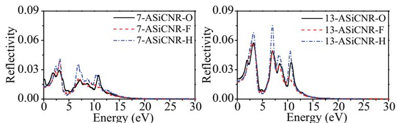
**Figure 9.** The theoretically calculated reflection spectra of 7- and 13-ASiCNRs terminated with O, F and H atoms.
