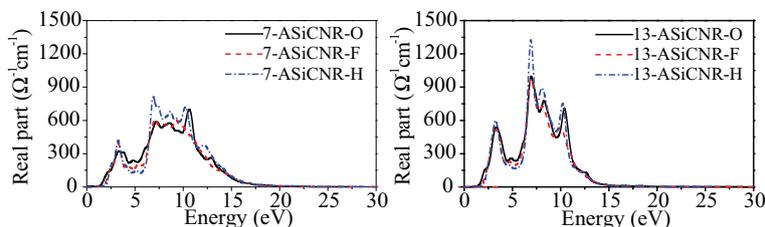
**Figure 11.** Real part of the conductance of O-, F- and H-terminated 7-ASiCNRs and 13-ASiCNRs. The black solid, red dashed and blue dashed dot lines indicate the conductance of O-, F- and H-terminated ASiCNRs, respectively.
