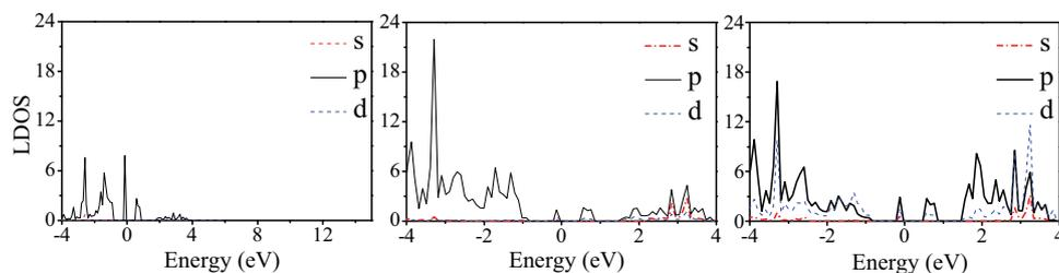
**Figure 5.** LDOS onto the (left) O atom, (centre) C atom and (right) Si atom of 13-ASiCNR-O.
