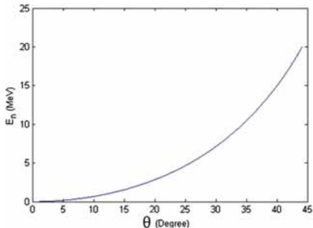
**Figure 3.** Neutron energy vs. scattering angle of the  $\alpha$ -particles.
