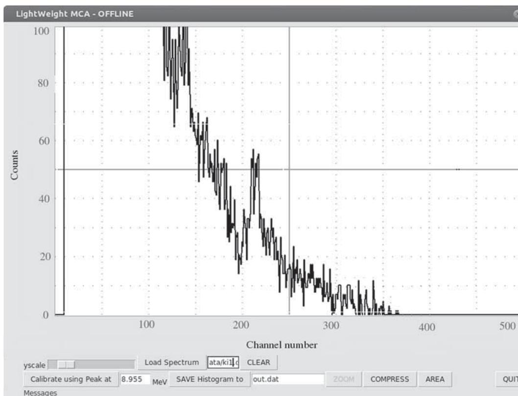
Figure 4. Spectrum from a KI sample, showing the 1.46 MeV  $\gamma$  line.
