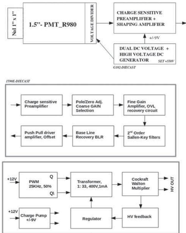
Figure 1. Block diagram of the signal processing electronics.
