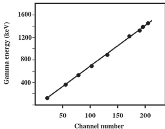
Figure 3. Energy calibration plot.
