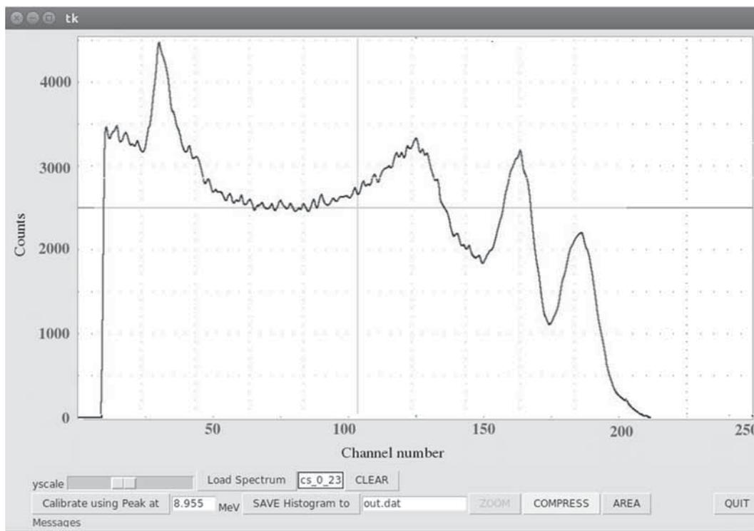
Figure 2. GUI window of the light weight MCA showing  $^{60}\text{Co}$  spectrum.
