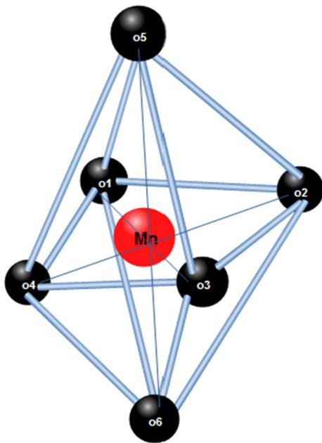
**Figure 2.** Manganese(II) distorted octahedron is expected to occupy any interstitial site. The  $z$ -axis is oriented transverse to the four tetragonal positions of oxygen atoms.
