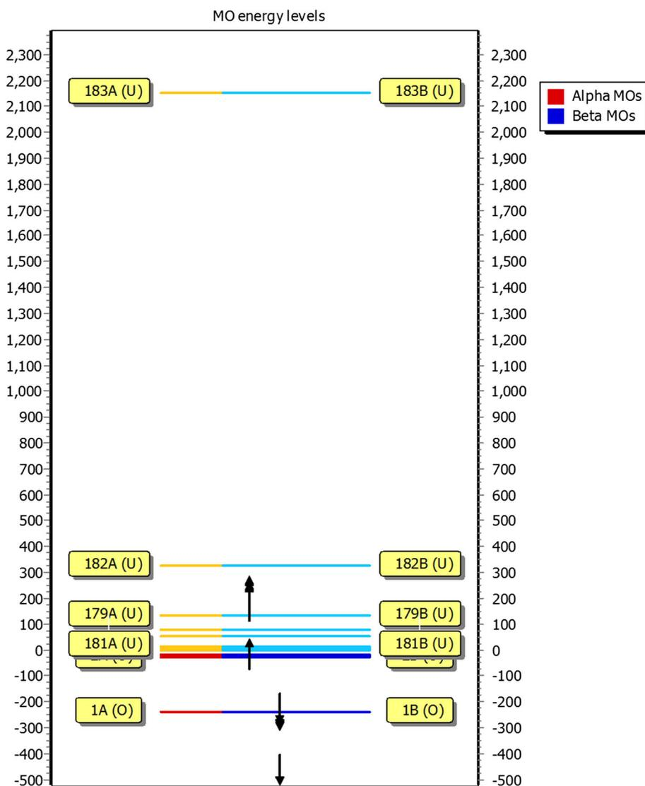
**Figure 5.** The molecular orbital energy level diagram for the dopant ion in the host DAMZ for the non-hybrid functional BP.
