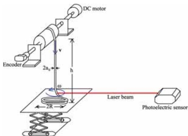
**Figure 1.** Experimental set-up is shown schematically. The rope with diameter  $2a_0$  is fed with uniform velocity  $v$  from the height  $h$  to the plane. It is laid down on the plane in a circular shape with the diameter  $2R$  and the angular velocity  $\omega = 2\pi f$ . The feeding velocity  $v$  is calculated from the radius of the cylinder and the frequency of the cylinder rotation measured by an encoder. The coiling frequency  $f$  is measured by a laser photoelectric sensor.
