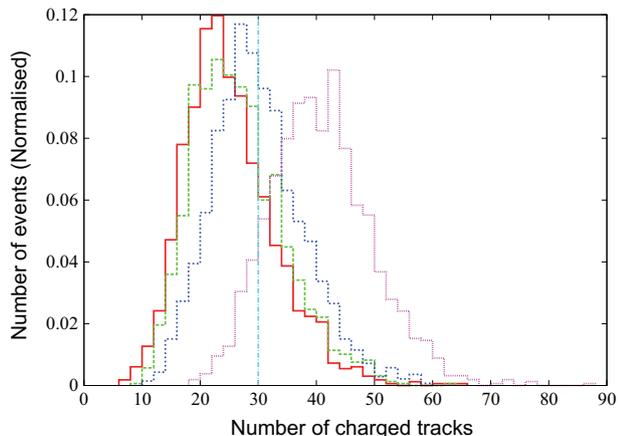
**Figure 2.** Normalized charge multiplicity distribution for the highest  $p_T$  jet formed by different ( $u\bar{u}$  – red,  $c\bar{c}$  – green,  $b\bar{b}$  – blue and  $g\bar{g}$  – violet) decay modes of the particle  $X$ .
