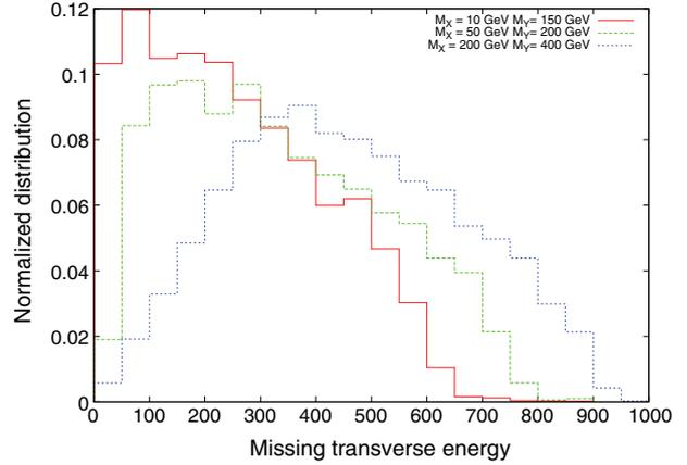
**Figure 9.**  $\cancel{E}_T$  distribution when  $X$  decays invisibly for three different sets of  $X$  and  $Y$  masses as shown in the inset.
