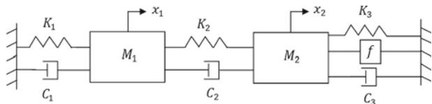
**Figure 1.** Schematic diagram of two-degrees of freedom spring-mass-damper system.
