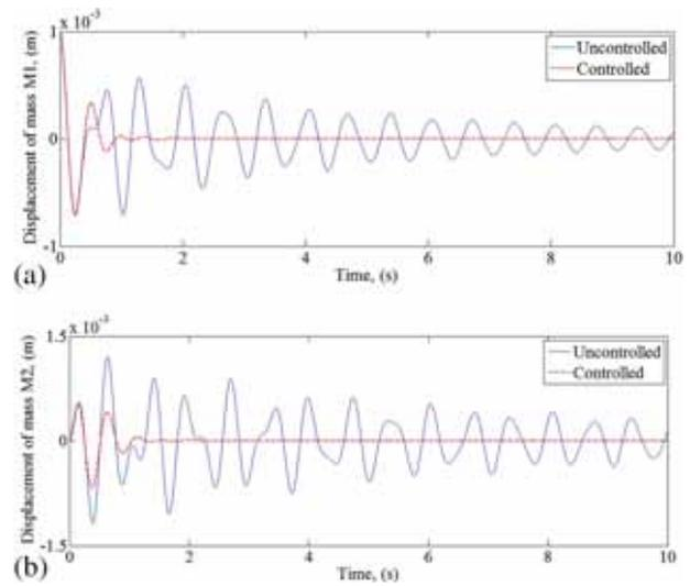
**Figure 4.** Uncontrolled/controlled time response of a two-degrees of freedom system.
