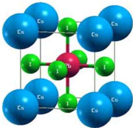
Figure 1. The unit cell of cubic CsPbI 3 .
