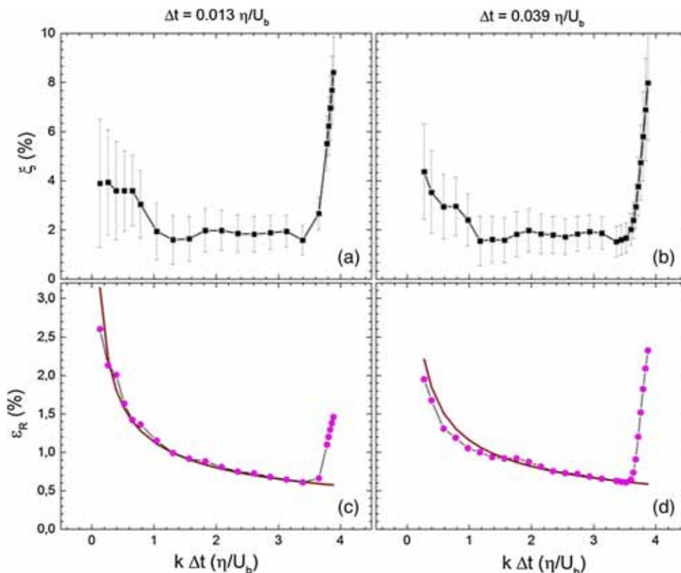
**Figure A1.** The fractional difference  $\xi$  defined by eq. (24) (panels **a** and **b**) and its error  $\varepsilon_R$  (panels **c** and **d**) vs. the interval of time-averaging ( $k\Delta t$ ) for two values of  $\Delta t$  (left and right columns). The curves without symbols in panels **c** and **d** represent the  $(k\Delta t)^{-1/2}$  dependence and has been adjusted to  $\varepsilon_R$  at some intermediate points. See parameters of the calculations in table B1.
