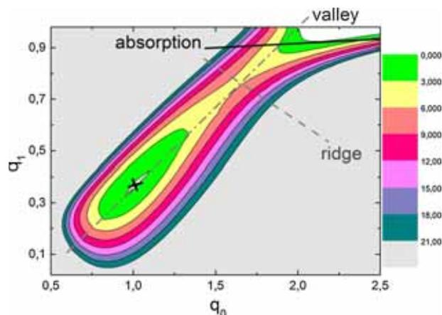
**Figure 2.** The realistic potential energy landscape for  $^{218}\text{Ra}$  along which the Brownian particle (fissioning nucleus) moves. The energy is calculated within the framework of the LSD model [31]. The ground state (cross), the ridge, the fission valley as well as the typical absorptive (scission) line are also shown.
