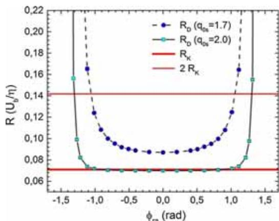
**Figure 9.** The dependence of the decay rates on the angle between the absorptive border and the ridge,  $\phi_{ra}$ , for the perpendicular valley for two values of  $q_{0s}$  indicated in the figure. Other notations are as in the previous figure. See parameters of the calculations in table B1.
