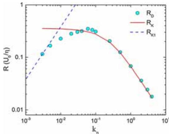
**Figure 11.** The dependence of the decay rates on the strength of friction  $k_\eta$  (see eq. (18)). Straight dash line indicates the 1D Kramers formula (25), and other notations are as in figures 8, 9, 10. See parameters of the calculations in table B1.
