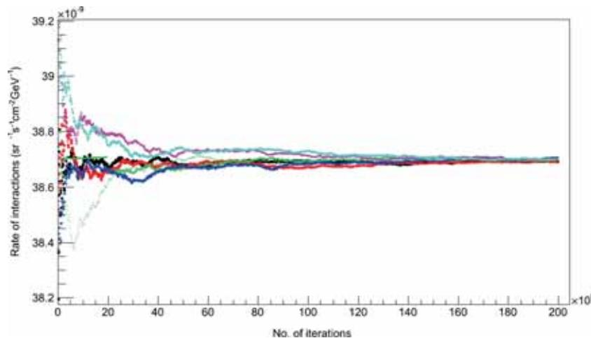
**Figure 11.** Expected flux rate for different number of iterations. The colours represent the execution of the program with different seeds of random number generation.
