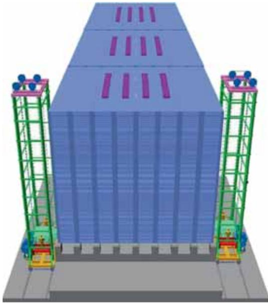
**Figure 1.** A schematic sketch of the INO ICAL detector.
