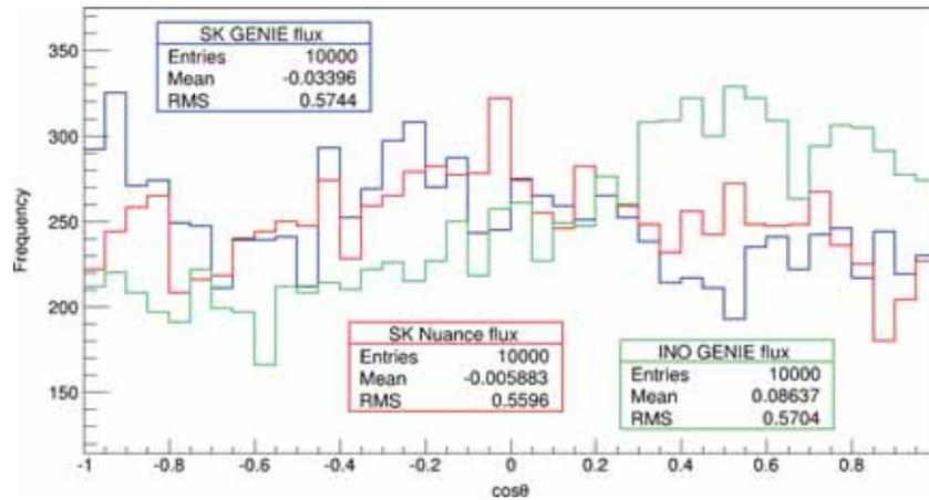
**Figure 9.** Comparison of the  $\cos\theta$  distributions of  $\nu_\mu$  at ICAL@INO with the 3D flux in the three different cases (mentioned above) in the energy range 0.1–10 GeV.
