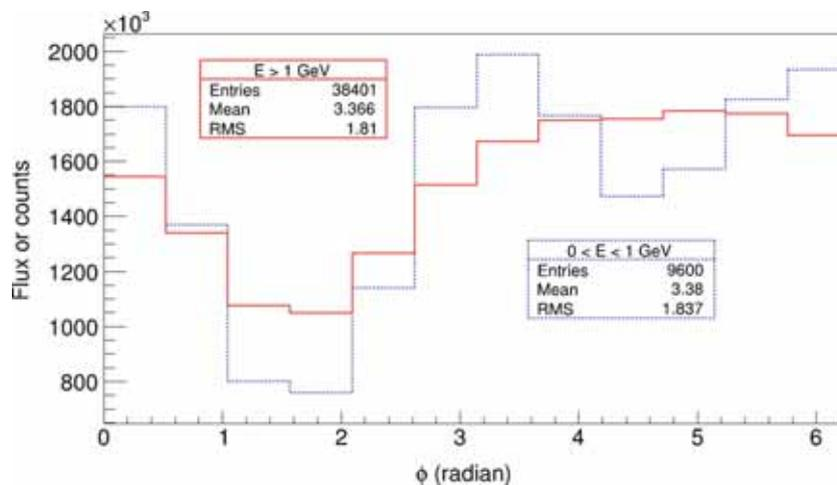
Figure 5. Azimuthal angle of incident neutrinos at ICAL@INO with the 3D flux at the INO site.
