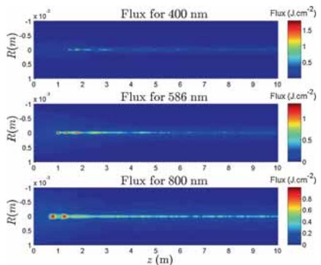
**Figure 2.** Evolution of the flux of laser pulses with the propagation distance  $z$ .
