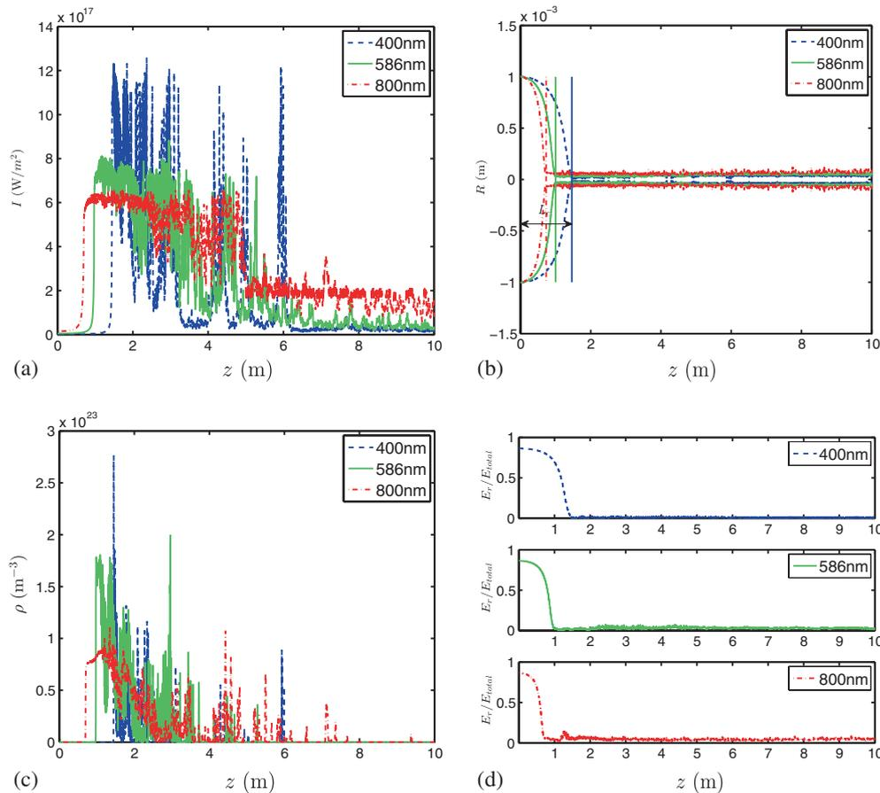
**Figure 1.** Evolution of the pulse and the on-axis electron density for different wavelengths with the propagation distance  $z$  for the same ratio of the incident power to  $P_{cr}$ . (a) The on-axis intensity of pulse; (b) beam radius; (c) the on-axis electron density; (d) the ratio of energy within the beam radius to the total energy.
