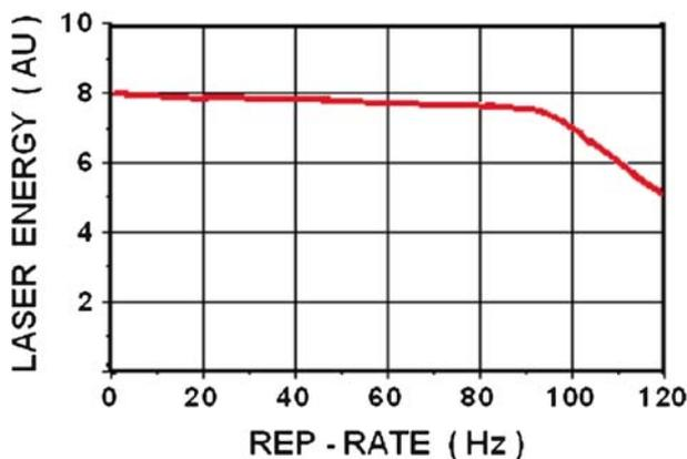
**Figure 9.** Performance characteristics of laser energy at different repetition rates.
