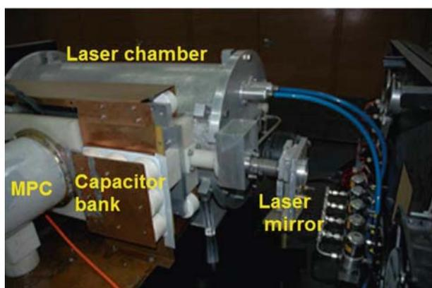
**Figure 1.** Repetitively pulsed XeCl excimer laser system with single-stage MPC.
