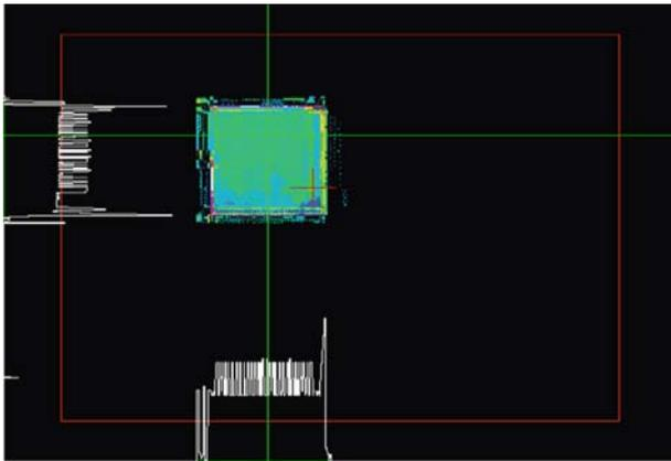
Figure 10. 2D beam profiles (flat-top).
