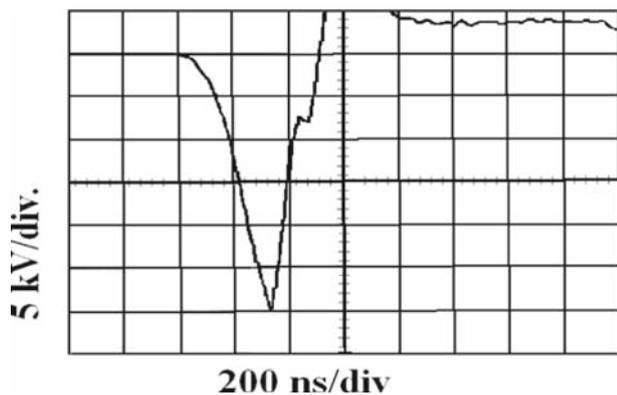
**Figure 6.** Charging voltage pulse of Cs (voltage rise time =  $\sim 260$  ns).
