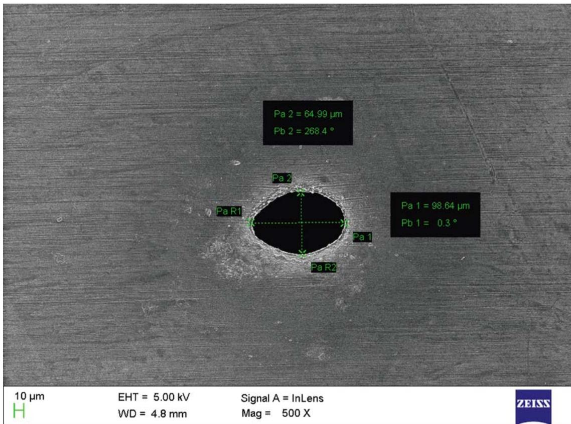
Figure 11. SEM image of the microhole generated with XeCl laser beam on a 0.2 mm thick copper sheet.
