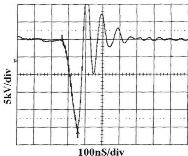
**Figure 7.** Discharge voltage pulse across the laser head (voltage rise time =  $\sim 100$  ns).
