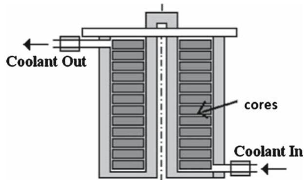
Figure 5. Schematic of the single-stage MPC with Ni-Zn toroidal cores.
