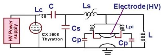
**Figure 2.** Single-stage MPC high voltage pulser for XeCl excimer laser.
