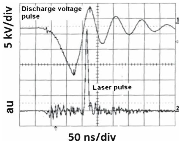
**Figure 8.** Typical discharge voltage pulse and the corresponding laser pulse.
