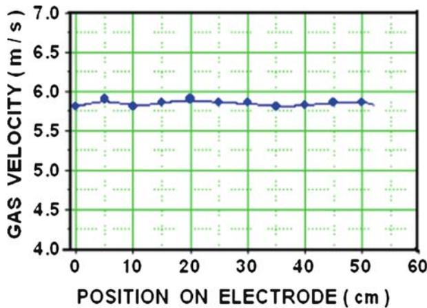
Figure 3. Gas flow velocity between the electrodes vs. position of electrode.
