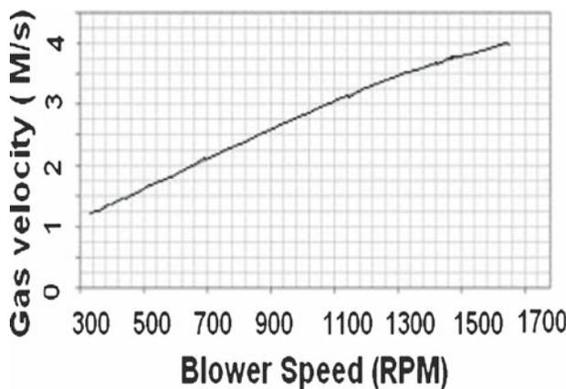
Figure 4. Velocity of the gas between the laser electrodes vs. blower speed.
