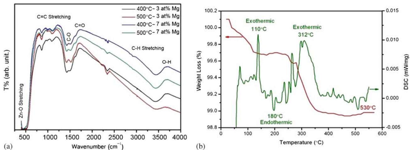
**Figure 2.** (a) FTIR spectra of Mg-doped ZnO nanoparticles annealed at 400 and 500°C and (b) DSC–TGA curves of 7 at% Mg-doped ZnO nanoparticles annealed at 400°C.
