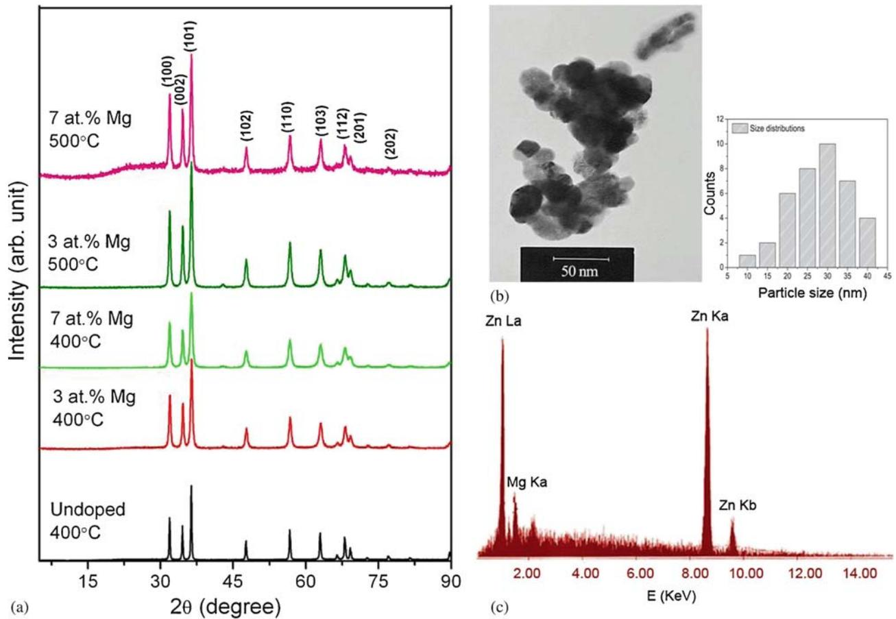
**Figure 1.** (a) XRD patterns of Mg-doped ZnO samples annealed at 400 and 500°C, (b) TEM image along with histogram indicating the size distribution of nanoparticles and (c) EDX spectrum for 7 at% Mg-doped ZnO nanopowder annealed at 400°C.
