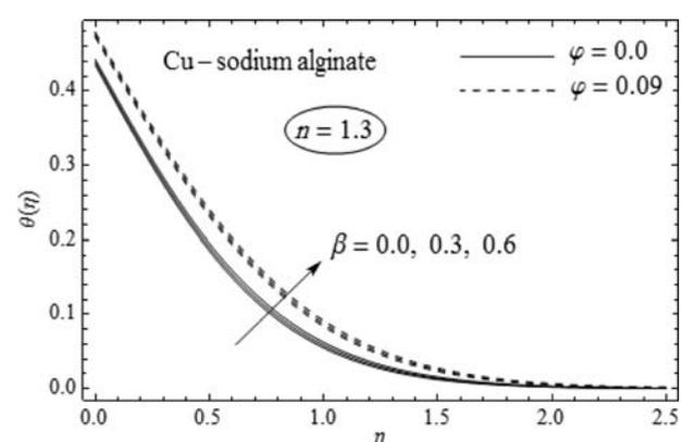
**Figure 5.** Temperature profiles for different values of  $\beta$  and  $\varphi$  with  $n = 1.3, Bi = 1$  and  $Pr_\infty = 5$ .
