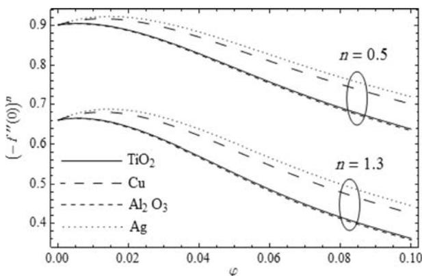
**Figure 11.** Variation of  $(-f''(0))^n$  with  $\varphi$  for different types of nanoparticles and  $n$  when  $\text{Bi} = 1$ ,  $\beta = 0.2$  and  $\text{Pr}_\infty = 5$ .
