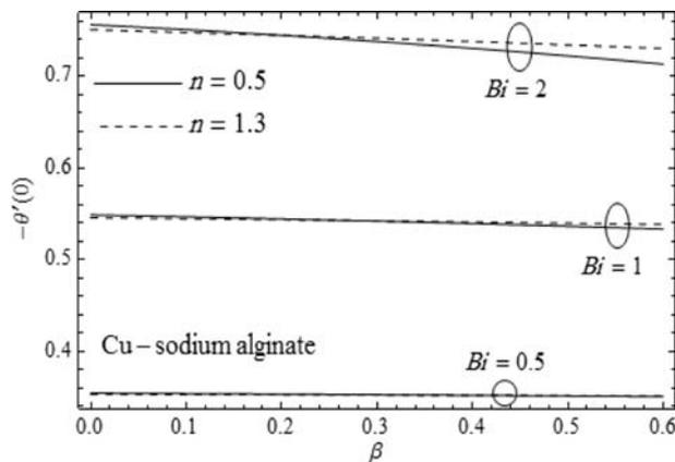
**Figure 15.** Variation of  $-\theta'(0)$  with  $\beta$  for different values of Bi and  $n$  when  $\varphi = 0.05$  and  $Pr_\infty = 5$ .
