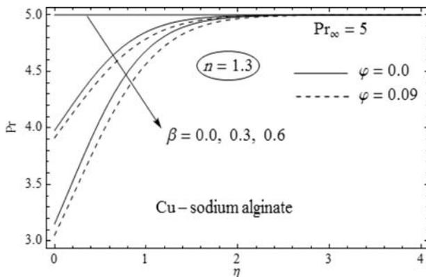
**Figure 6.** Variation of Prandtl number (Pr) for different values of  $\beta$  and  $\varphi$  with  $n = 1.3$  and  $Bi = 1$ .
