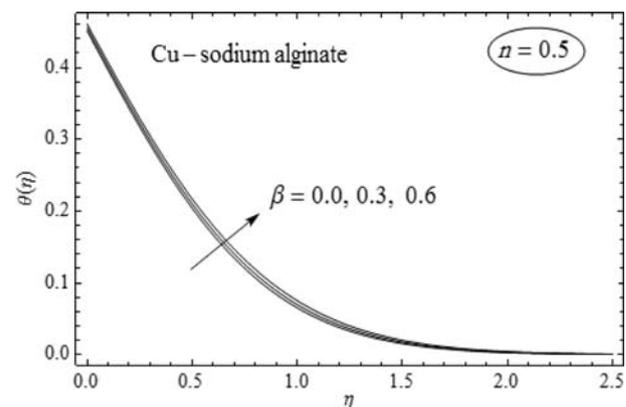
**Figure 9.** Temperature profiles for different values of  $\beta$  with  $n = 0.5$ ,  $\varphi = 0.05$ ,  $Bi = 1$  and  $Pr_\infty = 5$ .
