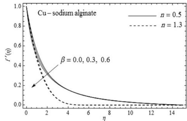
**Figure 8.** Velocity profiles for different values of  $\beta$  and  $n$  with  $\varphi = 0.05$ ,  $Bi = 1$  and  $Pr_\infty = 5$ .
