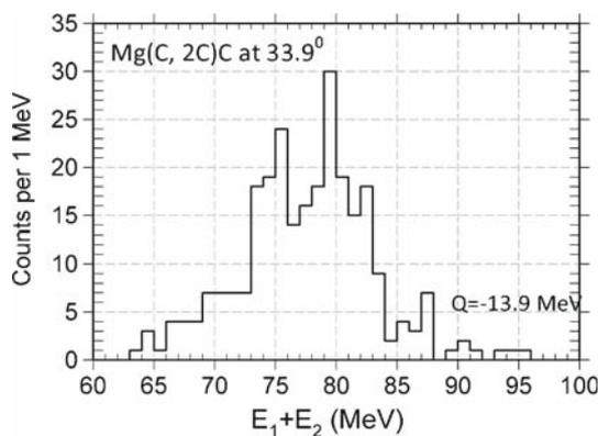
**Figure 6.** Summed energy spectrum for  $^{24}\text{Mg}(^{12}\text{C}, ^{212}\text{C})^{12}\text{C}$  reaction at  $\theta_1 = -\theta_2 = 33.9^\circ$  at 104 MeV. Counts around  $E_1 + E_2 \sim 90$  MeV belong to  $Q = -13.92$  MeV.
