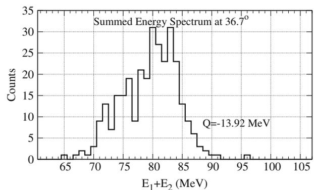
**Figure 8.** Summed energy spectrum for  $^{24}\text{Mg}(^{12}\text{C}, ^{212}\text{C})^{12}\text{C}$  reaction at  $\theta_1 = -\theta_2 = 36.7^\circ$  at 104 MeV. The counts around  $E_1 + E_2 \sim 90$  MeV belong to  $Q = -13.92$  MeV.
