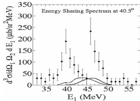
**Figure 4.** Energy sharing spectrum for the  $^{24}\text{Mg}(^{12}\text{C}, 2^{12}\text{C})^{12}\text{C}$  reaction at  $\theta_1 = -\theta_2 = 40.5^\circ$  at 104 MeV is compared with the normalized FR-DWIA predictions solid line and dotted line using repulsive core ( $R+A$ ) and all-through attractive ( $A$ ),  $^{12}\text{C}-^{12}\text{C}$  potentials respectively for the  $t$ -matrix generation.
