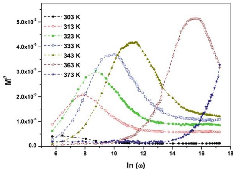
**Figure 10.** Temperature dependence of the dielectric modulus,  $M''(\omega)$ , for AMT at different frequencies.
