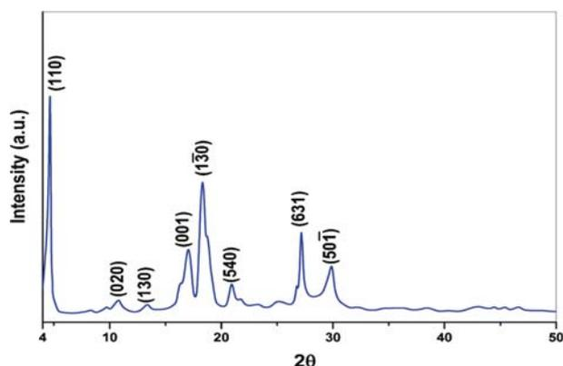
**Figure 1.** X-ray diffraction patterns of AMT in its powder form.
