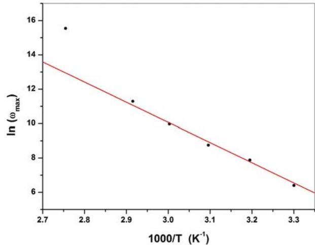
**Figure 11.** Temperature dependence of the frequency at the maximum  $M''(\omega)$ .
