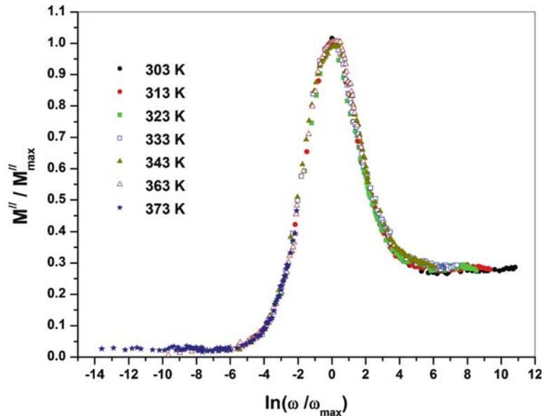
**Figure 12.** Variation of the normalized parameter  $M''/M''_{\max}$  as a function of  $\omega/\omega_{\max}$ .
