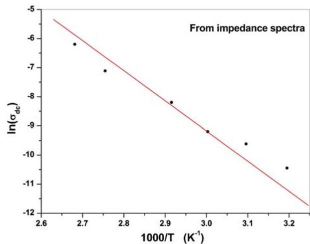
Figure 7. Temperature dependence of  $\sigma_{DC}$  for AMT.
