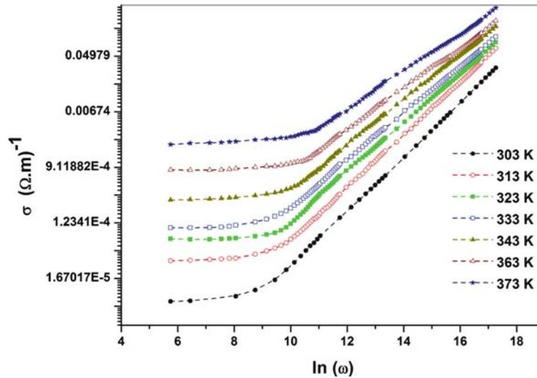
Figure 4. Frequency dependence of  $\ln \sigma(\omega, T)$  for AMT at different temperatures.
