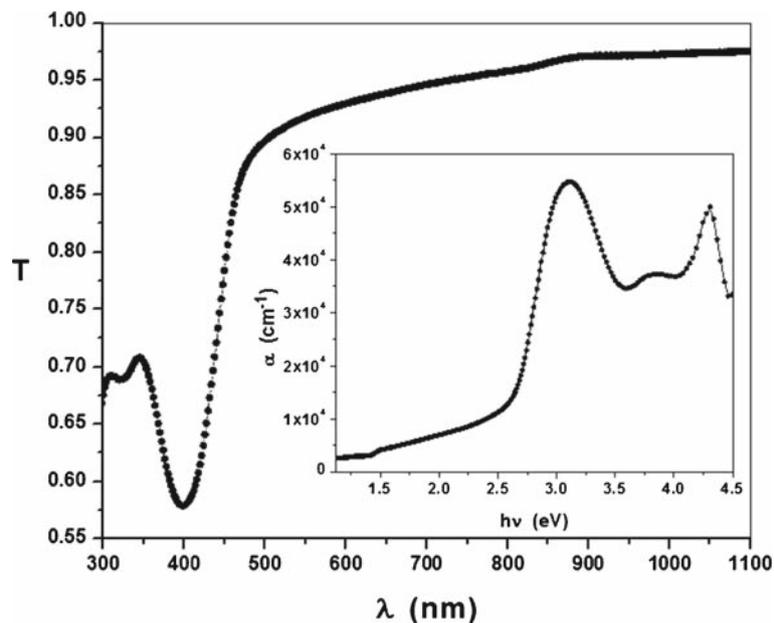
**Figure 13.** The spectral dependence of the normal incidence transmittance,  $T$ . The inset figure shows the spectral dependence of the absorption coefficient,  $\alpha$ .
