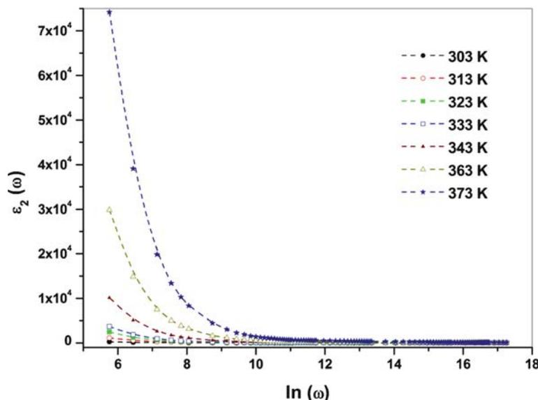
**Figure 9.** Frequency dependence of the dielectric loss,  $\varepsilon_2(\omega)$ , for AMT at different temperatures.
