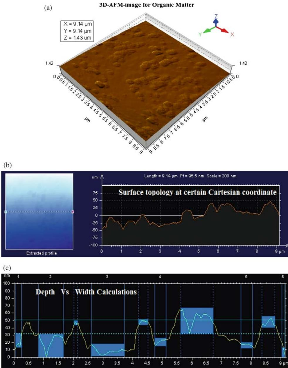
**Figure 3.** (a) 3D AFM-image captured for organic compound under investigations with Cartesian coordinate  $(x, y, z) = (9.14, 9.14, 1.43 \mu\text{m})$  respectively, (b) 2D AFM surface topology at certain  $(x-y)$  Cartesian coordinates and (c) AFM-computational calculations of depth vs. area of holes on the surface layer.
