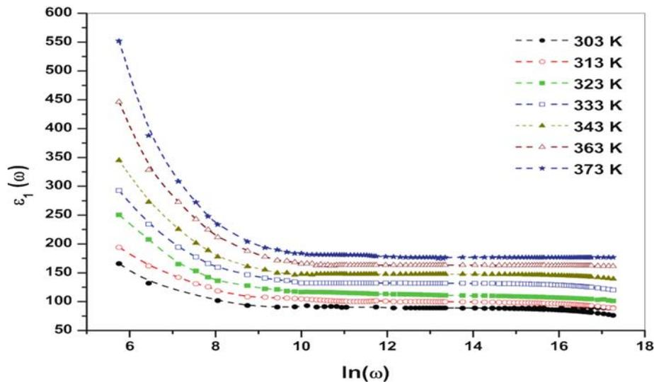
**Figure 8.** Frequency dependence of the dielectric constant,  $\varepsilon_1(\omega)$ , for AMT at different temperatures.
