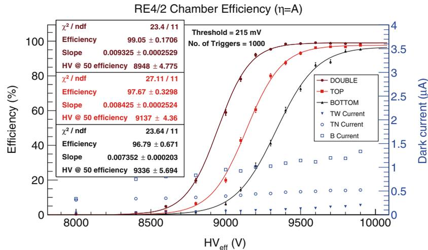
**Figure 7.** Sample efficiency plot for an RE4/2 RPC using the paddle covering the A section ( $\eta = A$ ), for the DOUBLE, TOP and BOTTOM configurations.
