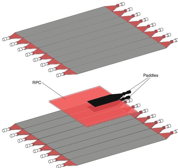
Figure 10. Glass RPC in the hodoscope.
