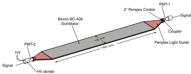
**Figure 1.** Schematic of a long scintillator paddle.
