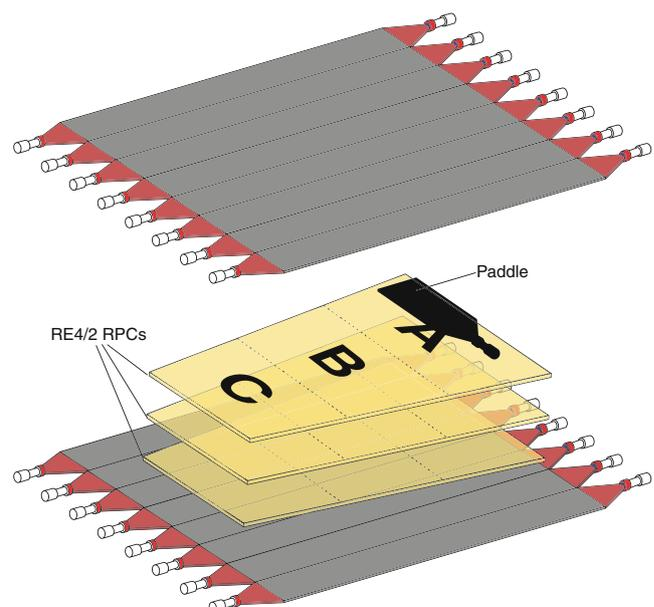
**Figure 6.** Geometry for the RE4/2 RPC.
