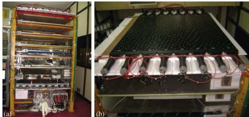
**Figure 2.** (a) The hodoscope and (b) the top plane having eight scintillators.
