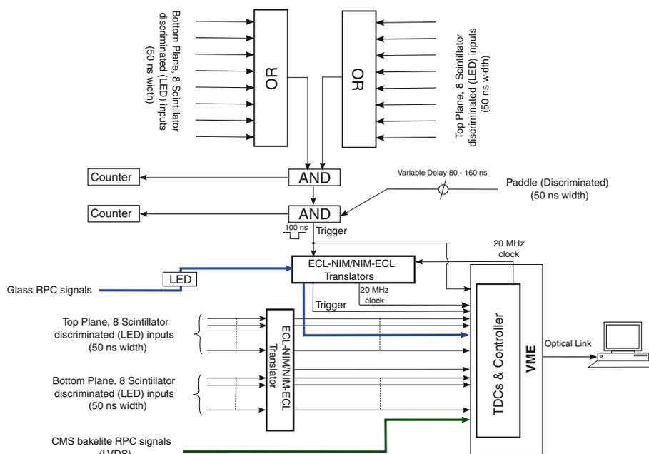
**Figure 3.** Block diagram of the hodoscope set-up.
