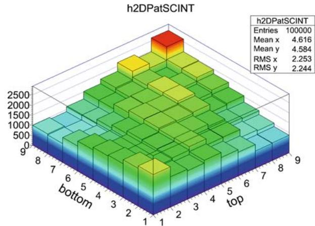
**Figure 4.** Coincidence plot of the top and bottom plane scintillators. Top 1–8 and bottom 1–8 are the numbers corresponding to the scintillators in the top and bottom planes of the hodoscope.
