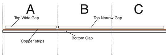
**Figure 5.** Side view of the RE4/2 RPC illustrating double layered gas gaps.
