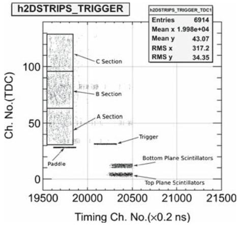
Figure 9. Timing distribution of signals.
