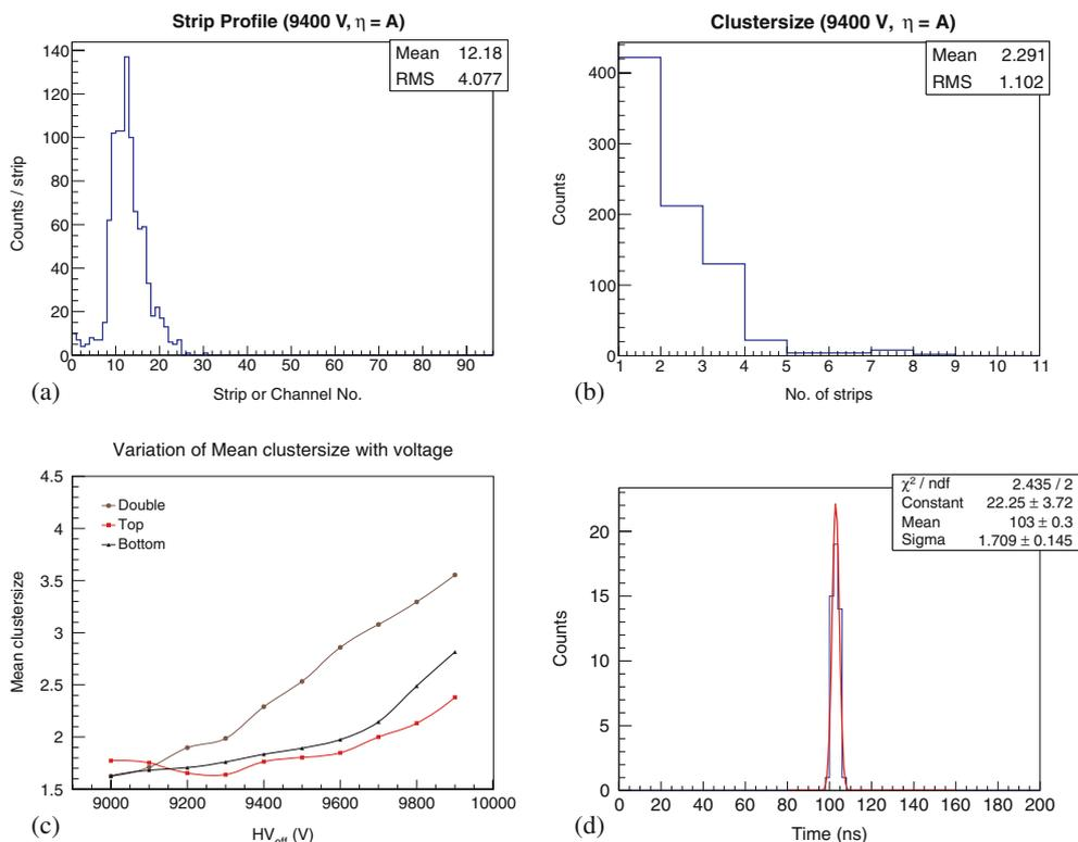
**Figure 8.** (a) Strip profile for the RPC at 9400 V ( $\eta = A$ , DOUBLE), (b) cluster size for the RPC at 9400 V ( $\eta = A$ , DOUBLE), (c) variation of mean cluster size with voltage and (d) distribution of the time interval between the signal of the 12th strip and the trigger. Plots shown are for  $\eta = A$  and DOUBLE configurations.
