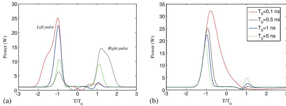
**Figure 3.** (a) Output pulse with various delay when  $T_0 = 1$  ns and  $\sim 40.3$  W input peak and (b) output pulse with various initial pulse width when the delay is  $-0.2T_0$  and the input peak is  $\sim 40.3$  W.
