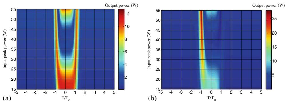
**Figure 4.** Pulse evolution against various input peak power for a delay of (a)  $235$  ps and (b)  $-235$  ps.
