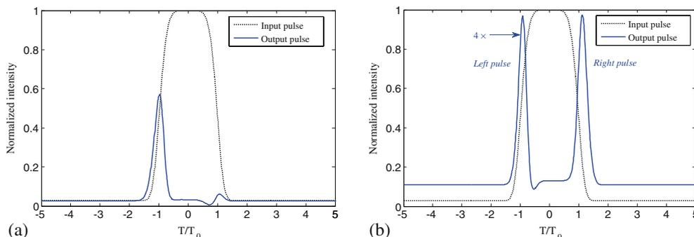
**Figure 2.** (a) Output single pulse with  $-235$  ps delay and (b) output double-pulse with  $235$  ps delay.
