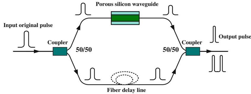
**Figure 1.** Schematic diagram of the proposed device for pulse generation and compression.
