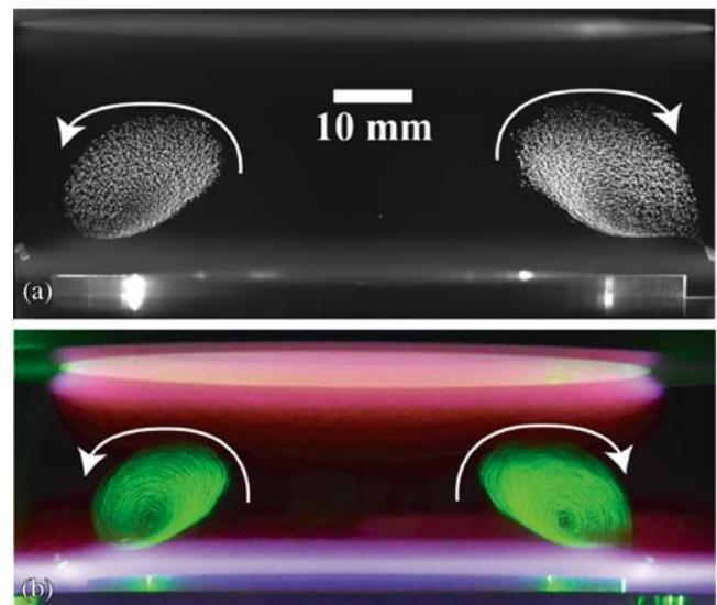
**Figure 5.** Two poloidal planes of the dust torus when illuminated using a vertical laser sheet along torus diameter taken (a) with help of a sCMOS camera and (b) with a visible DSLR camera.
