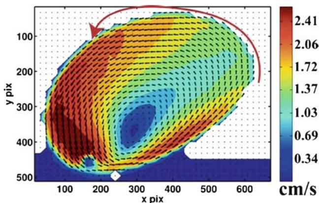
**Figure 6.** The velocity profile of the dust particles as an ensemble average of 479 flow fields obtained from PIV analysis with an interrogation window size of  $32 \times 32$  at 50% overlap at 10.1 ms exposure time in one poloidal plane of the dust torus. The colour bar represents the magnitudes of dust velocities and the direction of arrows represents the direction of dust rotation.
