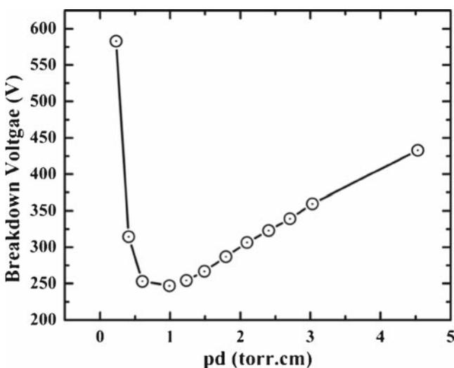
**Figure 2.** Paschen curve obtained in the present set-up at an interelectrode separation of 4 cm.
