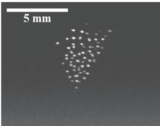
**Figure 4.** The image showing the vertical view of three-dimensional dust structures taken with the help of sCMOS camera.
