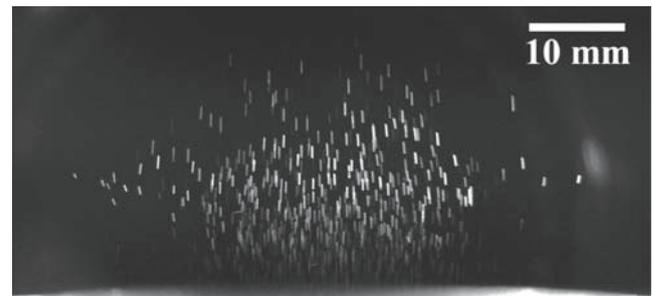
**Figure 3.** High-amplitude dust oscillations at very low pressures ( $\sim 20 \text{ Pa}$ ).
