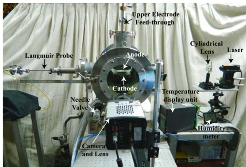
**Figure 1.** Photograph of the experimental set-up with different subparts.
