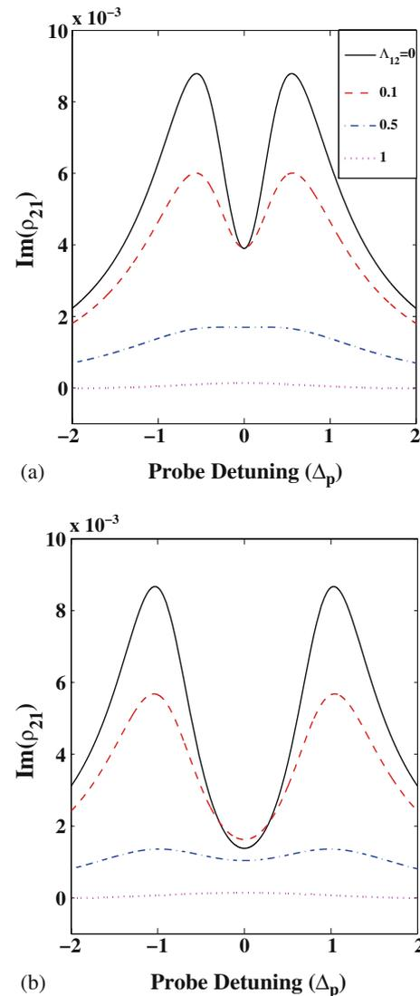
**Figure 2.** Imaginary part of  $\rho_{21}$ . (a)  $\Omega_c = 0.5$  and (b)  $\Omega_c = 1$  for unequal spontaneous emission rates  $\gamma_{32} = 0.16$ . The values of incoherent pumping  $\Lambda_{12}$  for each curve are shown in the legend. The probe field Rabi frequency  $\Omega_p = 0.01$ . All parameters ( $\Delta_p$ ,  $\Omega_c$ ,  $\Omega_p$ ,  $\gamma_{32}$  and  $\Lambda_{12}$ ) used here and in subsequent figures are in units of  $\gamma_{21}$ .
