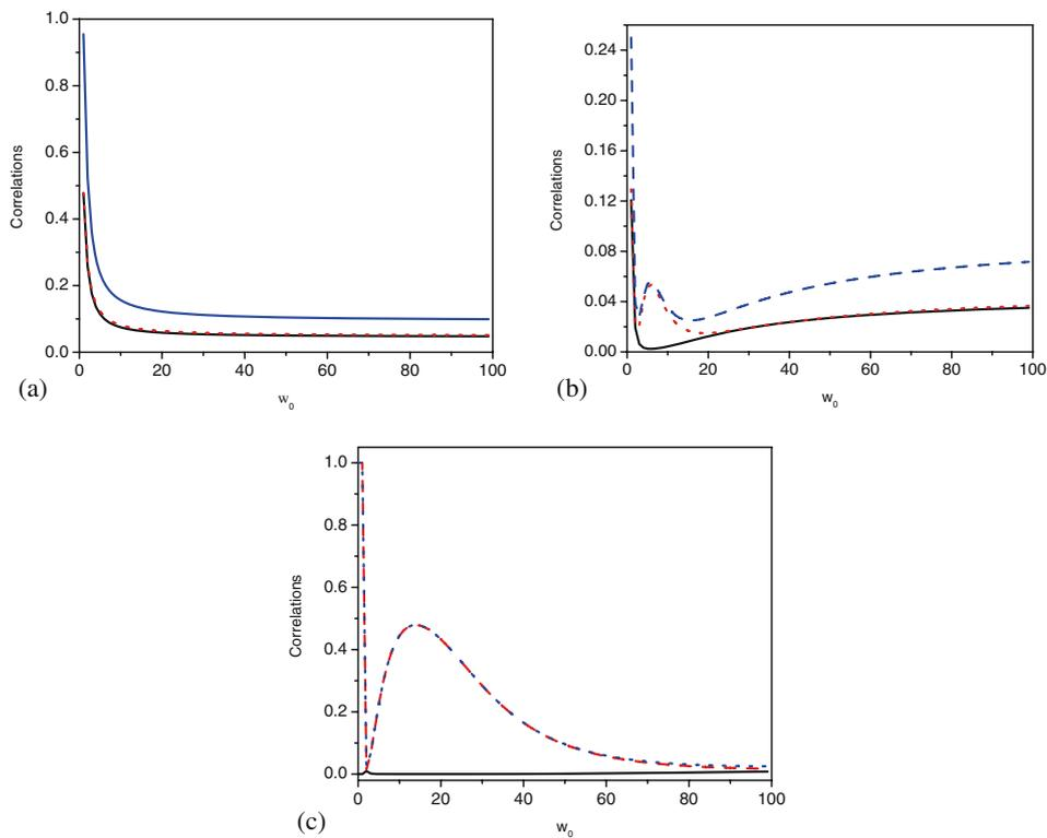
**Figure 3.** The three types of correlations are plotted against the size of wave packet  $W$  with rapidity  $\alpha = 300$ . In each of these figures, the black curve represents classical correlations, red is for quantum discord and the blue stands for quantum mutual information. The value of  $K$  in each figure is: (a)  $K = 0.01$ , (b)  $K = 10$  and (c)  $K = 100$ .
