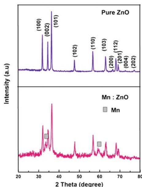
**Figure 1.** XRD pattern of synthesized pure ZnO and Mn-doped ZnO nanoparticles.
