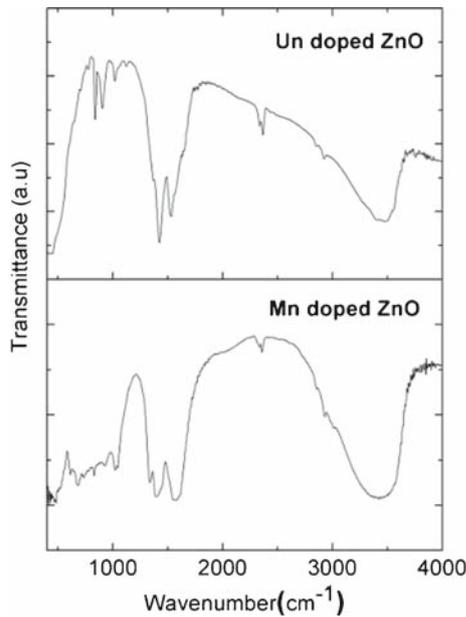
**Figure 5.** FTIR spectra of (a) pure ZnO and (b) Mn-doped ZnO at room temperature.
