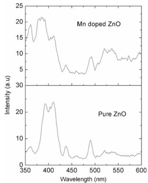
**Figure 6.** Photoluminescence spectra of pure ZnO and Mn-doped ZnO under an excitation wavelength of 325 nm at room temperature.
