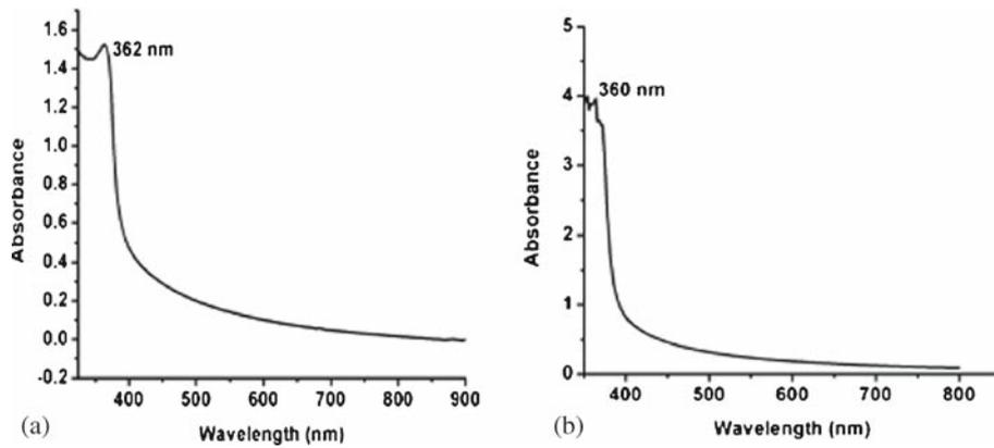
**Figure 3.** Absorption spectra of pure and Mn-doped ZnO nanoparticles.
