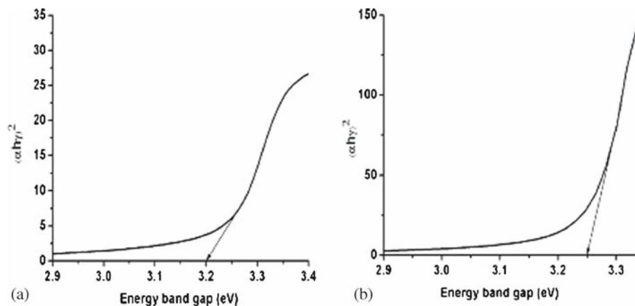
**Figure 4.** The plot of  $(\alpha hv)^2$  vs.  $hv$  for (a) pure ZnO and (b) Mn-doped ZnO nanoparticles.
