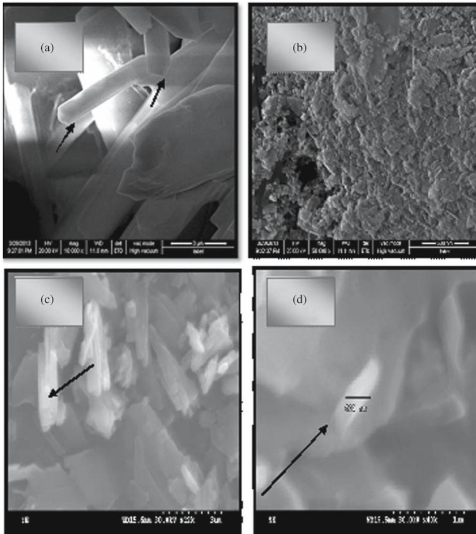
**Figure 2.** (a) and (b) show SEM images for rod-shaped pure ZnO and (c) and (d) show Mn-doped ZnO nanoparticle.
