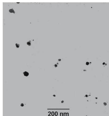
**Figure 5.** TEM image of silver nanoparticles.
