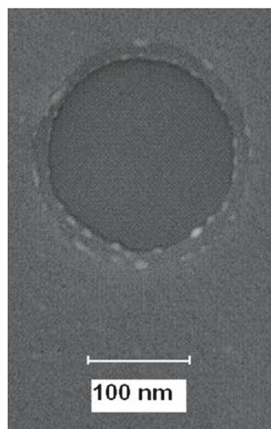
**Figure 8.** TEM image of silver nanoparticles-decorated PDA nanovesicles.
