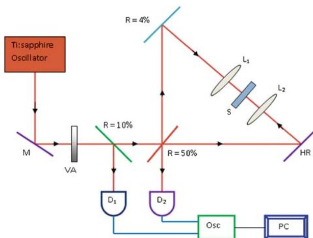
**Figure 10.** ARINS experimental set-up. M – mirror,  $L_1$ ,  $L_2$  – lenses, HR – high reflectivity mirror, S – sample, VA – variable attenuator,  $D_1$ ,  $D_2$  – detectors, Osc – digital oscilloscope, PC – computer.
