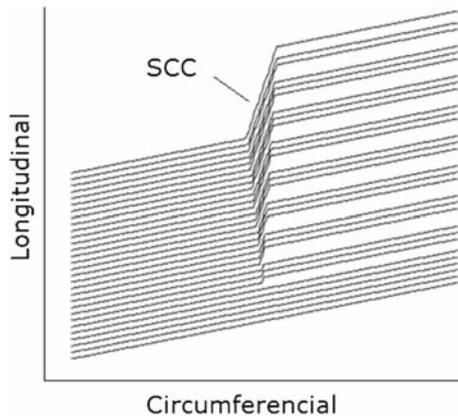
**Figure 2.** Two-dimensional displacement on the pipe surface.
