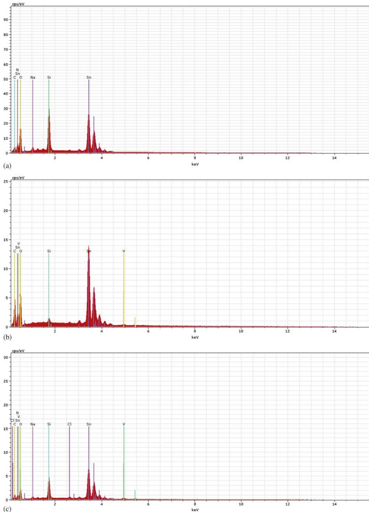
**Figure 3.** Energy-dispersive X-ray analysis spectra of pure and V-doped SnO<sub>2</sub> thin films: (a) undoped SnO<sub>2</sub>, (b) 5% V-doped SnO<sub>2</sub> and (c) 10% V-doped SnO<sub>2</sub>.
