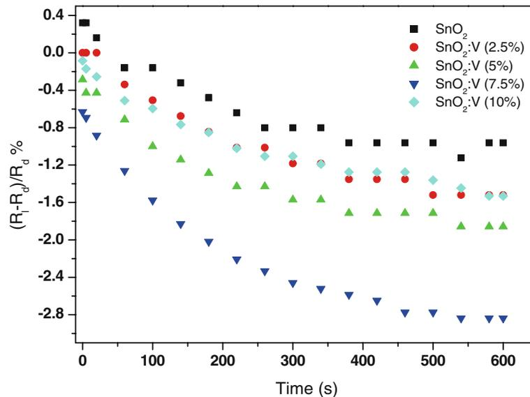
**Figure 11.** The variation of  $S\% = ((R_1 - R_d)/R_d) \times 100$  with time of SnO<sub>2</sub>:V thin films for different doping levels (at% in solution).
