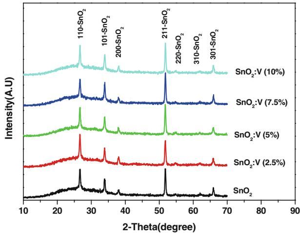
**Figure 1.** XRD patterns of SnO<sub>2</sub>:V thin films for different doping levels.
