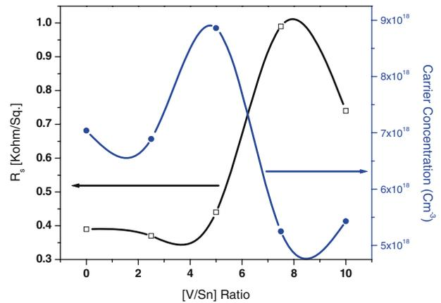
**Figure 7.** The variation in sheet resistance and carrier concentration of SnO<sub>2</sub>:V thin films for different doping level [V/Sn] ratios.
