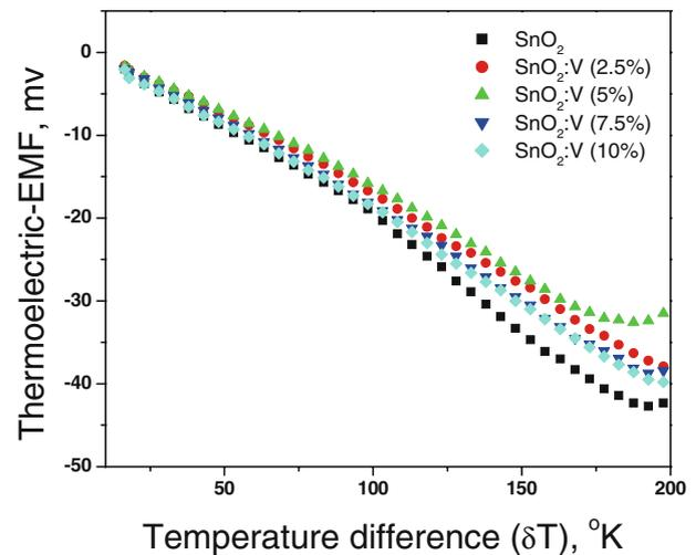
**Figure 9.** The variation in thermoelectric-EMF with temperature difference of  $\text{SnO}_2:\text{V}$  thin films for different doping levels.
