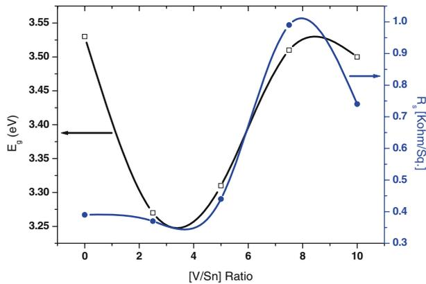
**Figure 8.** The variation in sheet resistance and optical direct band gap of  $\text{SnO}_2:\text{V}$  thin films for different doping level  $[\text{V}/\text{Sn}]$  ratios.
