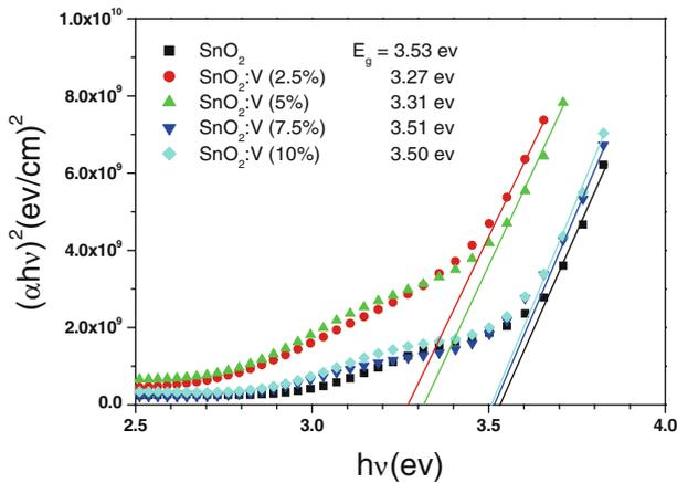
**Figure 6.** Plots of  $(\alpha hv)^2$  vs.  $(hv)$  for SnO<sub>2</sub>:V thin films for different doping levels.
