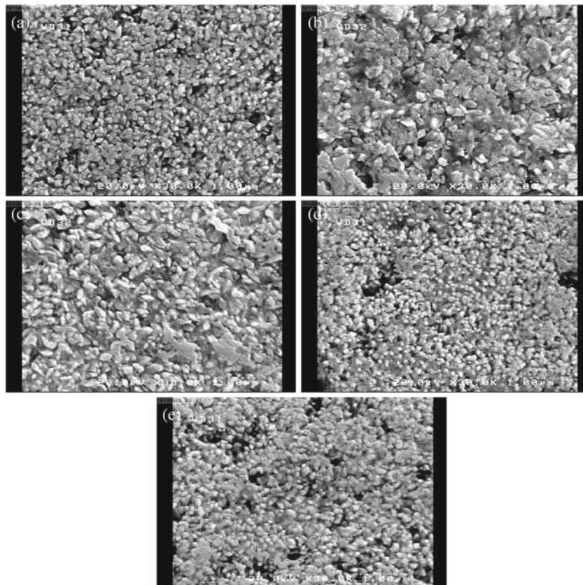
**Figure 2.** FESEM images of SnO<sub>2</sub>:V films for different V-content: (a) 0, (b) 2.5, (c) 5, (d) 7.5 and (e) 10 at%.
