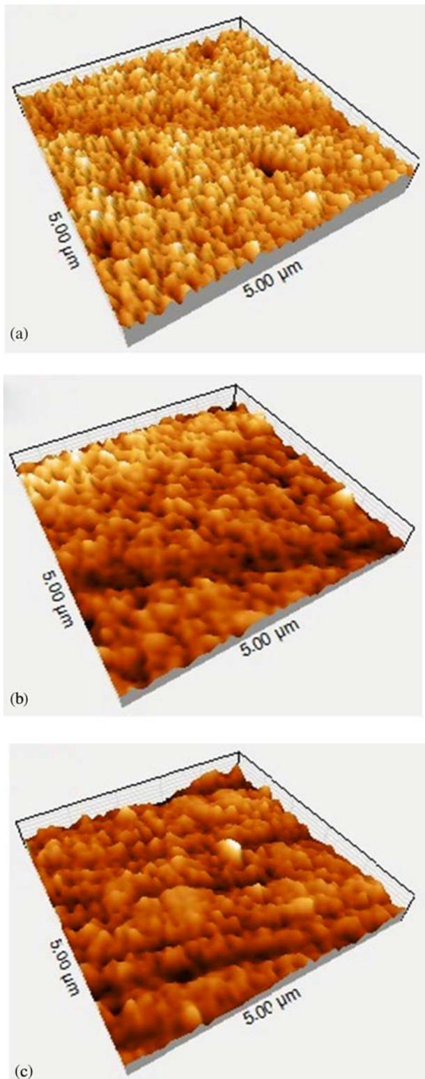
**Figure 4.** AFM images of  $\text{SnO}_2:\text{V}$  films for different V-content: (a) 0, (b) 5 and (c) 10 at%.
