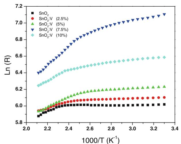
**Figure 10.** The variation in resistance with temperature of  $\text{SnO}_2:\text{V}$  thin films for different doping levels.
