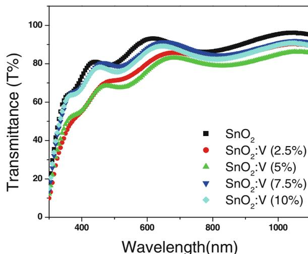
**Figure 5.** The variation of transmittance with the wavelength of  $\text{SnO}_2:\text{V}$  thin films for different doping levels.
