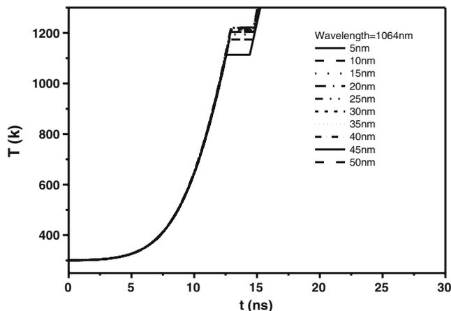
**Figure 8.** Temperature of silver nanoparticles under irradiation of Nd:YAG laser at 1064 nm wavelength with respect to the effect of size on the melting temperature of nanoparticles.
