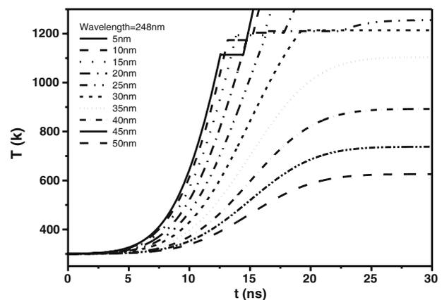
**Figure 2.** Temperature of silver nanoparticles under the irradiation of excimer laser at a wavelength of 248 nm with respect to the effect of size on the melting temperature of the nanoparticles.
