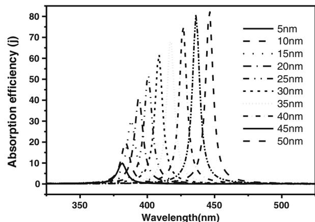
**Figure 1.** Absorption spectra for spherical silver nanoparticles with radii between 5 and 50 nm.
