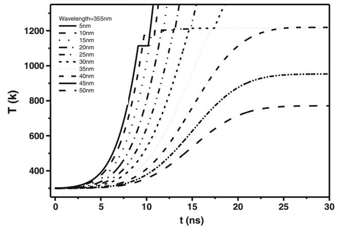
**Figure 5.** Temperature of silver nanoparticles under intermediate intensity irradiation of third harmonic of Nd:YAG laser at 355 nm wavelength with respect to the effect of size on the melting temperature of the nanoparticles.
