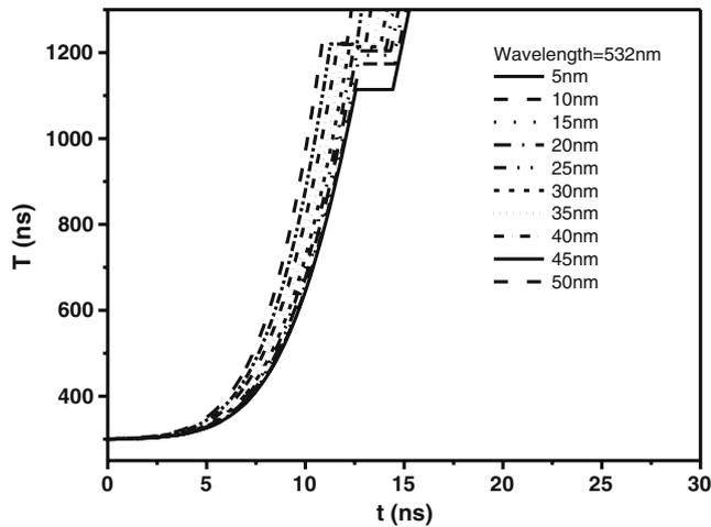
**Figure 7.** Temperature of silver nanoparticles under irradiation of second harmonic of Nd:YAG laser at 532 nm wavelength with respect to the effect of size on the melting temperature of the nanoparticles.
