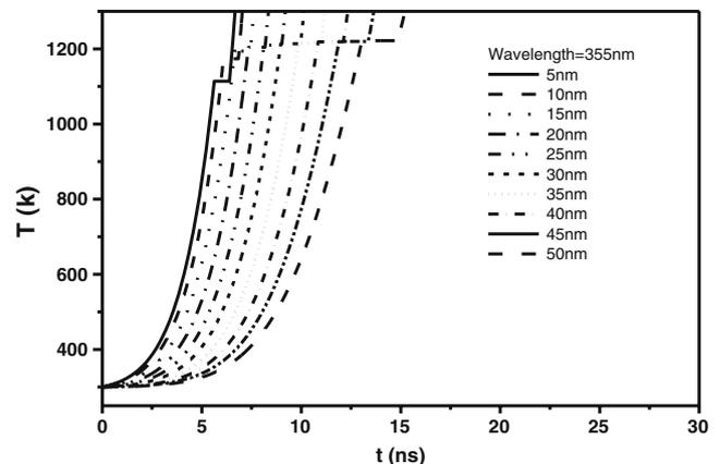
**Figure 6.** Temperature of silver nanoparticles under high intensity irradiation of third harmonic of Nd:YAG laser at 355 nm wavelength with respect to the effect of size on the melting temperature of the nanoparticles.
