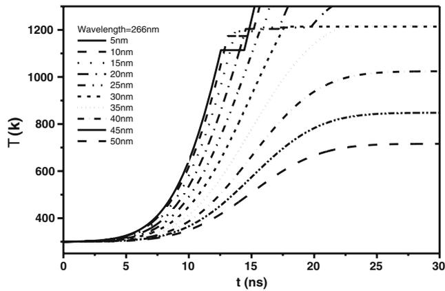
**Figure 3.** Temperature of silver nanoparticles under fourth harmonic of Nd:YAG laser irradiation at 266 nm wavelength with respect to effect of size on the melting temperature of the nanoparticles.
