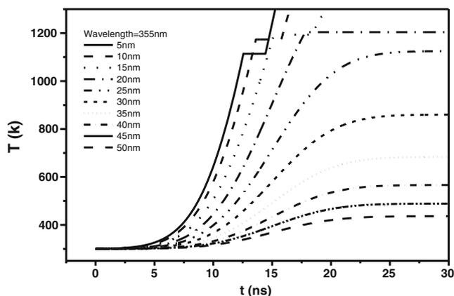
**Figure 4.** Temperature of silver nanoparticles under low intensity irradiation of third harmonic of Nd:YAG laser at 355 nm wavelength with respect to the effect of size on the melting temperature of the nanoparticles.
