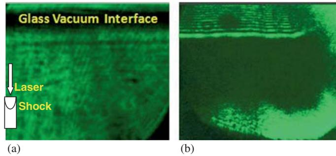
**Figure 4.** Typical shadowgram (a) without shock and (b) with shock wave propagation.
