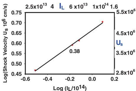
**Figure 6.** The scaling of the shock velocity and the shock pressure with laser intensity.
