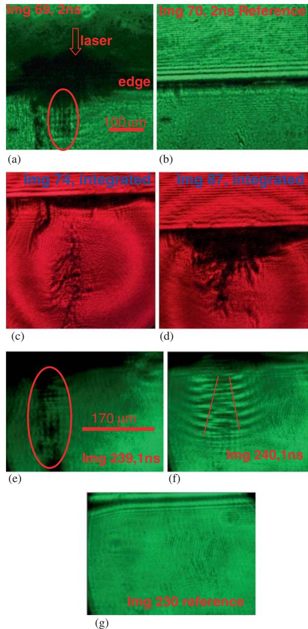
**Figure 7.** (a) Shadowgram showing jet-like structures after a delay of 2 ns; (b) a reference shadowgram taken in the absence of plasma (shock); (c), (d) time-integrated shadowgrams with a He–Ne laser, much after the experiment; (e) shadowgram after 1 ns delay; (f) shadowgram showing diverging trend in the structure; (g) reference shadowgram taken in the absence of plasma (shock).
