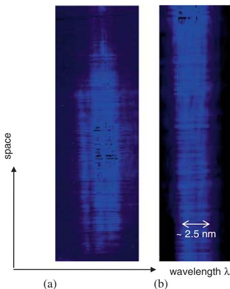
**Figure 2.** Typical shadowgram (a) with and (b) without shock wave propagation. Shock is propagating downwards.
