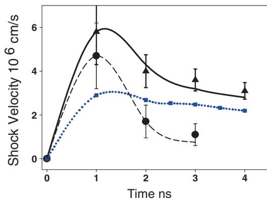
**Figure 5.** Variation of the shock velocity with time at two laser intensities:  $4 \times 10^{13}$  (filled circles, dashed curve) and  $10^{14}$  W/cm<sup>2</sup> (triangles, solid curve). The curves are only to guide the eyes. Also shown is the simulated velocity profile using MULTI code (squares, dotted curve) for  $10^{14}$  W/cm<sup>2</sup>.
