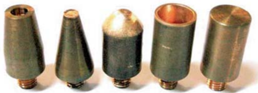
Figure 4. Different types of anode inserts in this study (right to left): cylindrical with flat top, cylindrical with hollow top, spherical with convex top, cone with flat top, and cone with hollow top.
