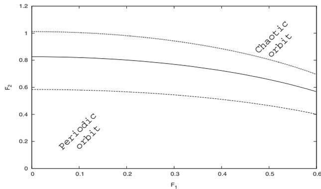
**Figure 1.** Minimum value of  $F_2$  required to suppress chaos for various amplitudes  $F_1$  using power average method for four cases, namely cosine force with phase (solid line), square force (short dashed line), sawtooth force (long dashed line), triangular force (long dashed line) as second harmonic excitations.
