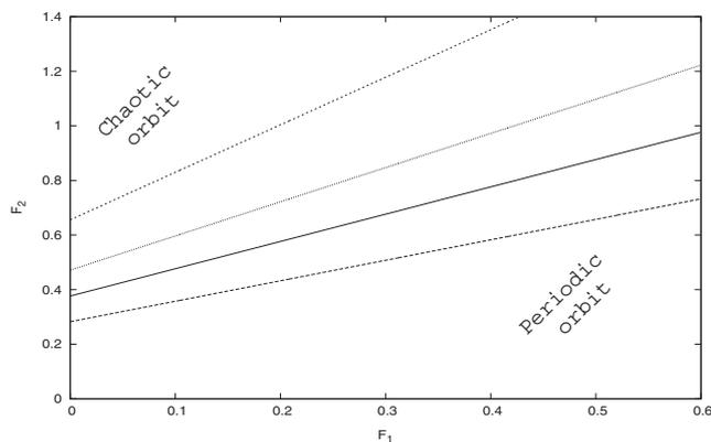
**Figure 2.** Threshold value of  $F_2$  required to suppress chaos for various amplitudes  $F_1$  using Melnikov method for four cases, namely cosine force with phase (solid line), square force (dashed line), sawtooth force (dotted line), triangular force (dash with dotted line) as second harmonic excitations.
