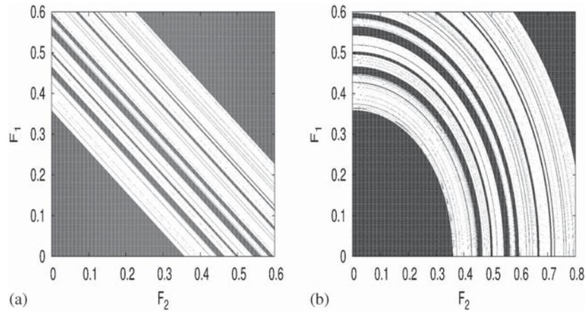
**Figure 3.** Phase diagram of eq. (4) for the cosine periodic force at the main harmonic resonance (black dot represents periodic region and white space represents chaotic region). (a) Cosine force without phase ( $\psi = 0$ ) and (b) cosine force with phase ( $\psi = 1.5844$ ) as second harmonic excitations.
