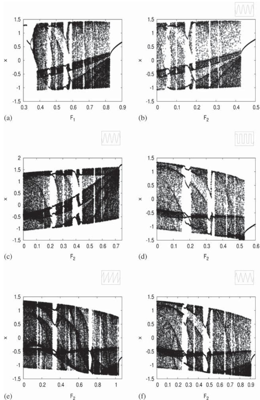
**Figure 5.** Bifurcation diagram of eq. (4) for various periodic forces as second harmonic at the main resonance. (a) Bifurcation diagram in the absence of second harmonic excitations, (b) cosine force without phase, (c) cosine force with phase, (d) square force, (e) sawtooth force and (f) triangular force as second harmonic excitations.
