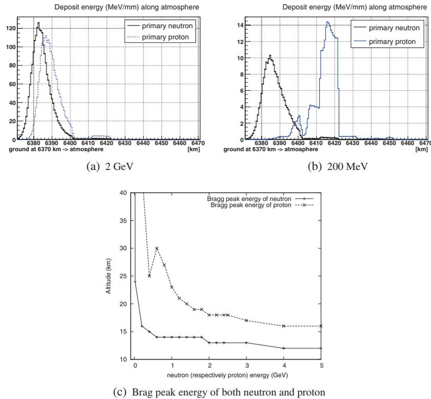
**Figure 3.** Plot of the differential deposit energy of protons vs. the depth in the Earth’s atmosphere. The Earth’s magnetic field is assumed to be  $47\mu T$ .
