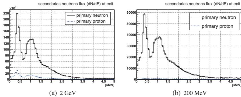
**Figure 4.** Spectrum of secondary neutrons in the atmosphere.
