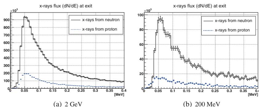
**Figure 5.** Yield of X-rays from neutron and proton in the atmosphere.
