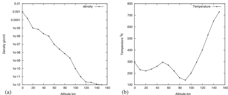
**Figure 2.** (a) Atmosphere mass density and (b) temperature using the NRLMSISE standard atmosphere model.
