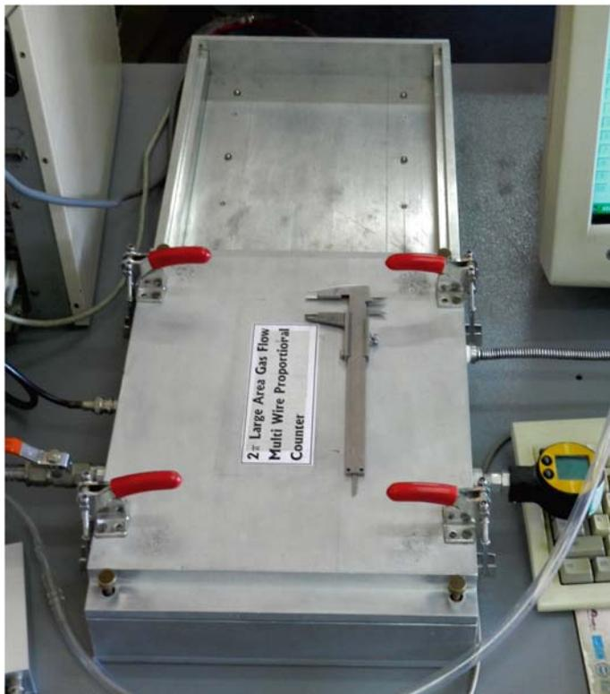
**Figure 4.** Completely assembled  $2\pi$ - $\beta$  chamber in operation with vacuum accessories.
