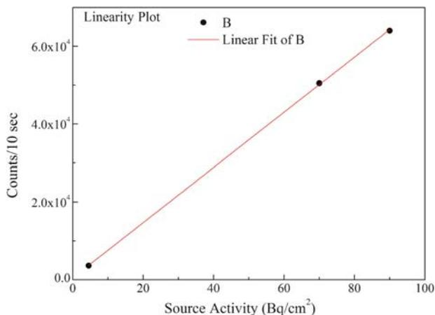
**Figure 11.** Linearity plot of counts vs. source activity.
