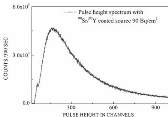
**Figure 9.** Pulse height spectrum of the PC with the  $^{90}\text{Sr}/^{90}\text{Y}$  source no. 7400.
