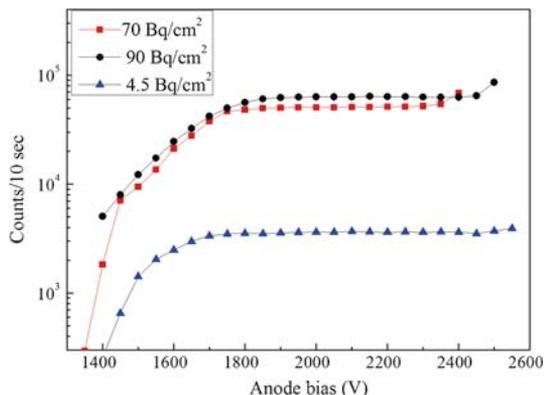
**Figure 10.** Voltage counting curve using the  $^{90}\text{Sr}/^{90}\text{Y}$  coated sources of various activities.
