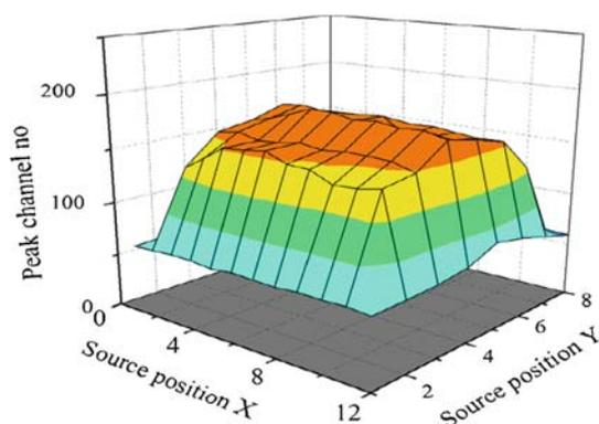
**Figure 7.** Pulse height variation profile over the sensitive region covered by the collimator window.
