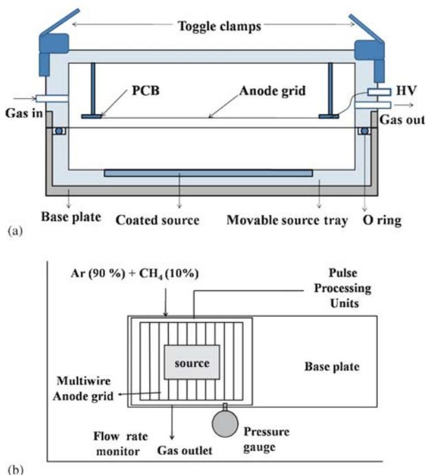
**Figure 3.** Schematic of MWPC. (a) Side section view of the PC structure and (b) PC with accessories.
