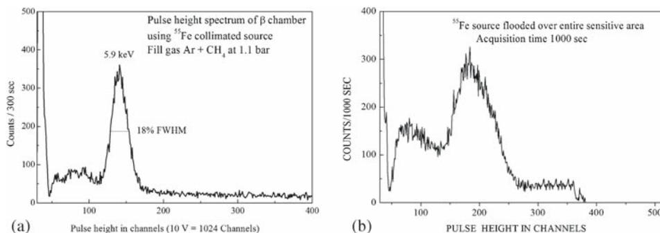
**Figure 8.** Pulse height spectra with  $^{55}\text{Fe}$  source placed at (a) collimator aligned with the anode wire and (b) flooded over the entire sensitive region of the chamber.
