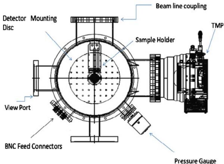
**Figure 1.** Schematic view of general-purpose scattering chamber facility at IPR.
