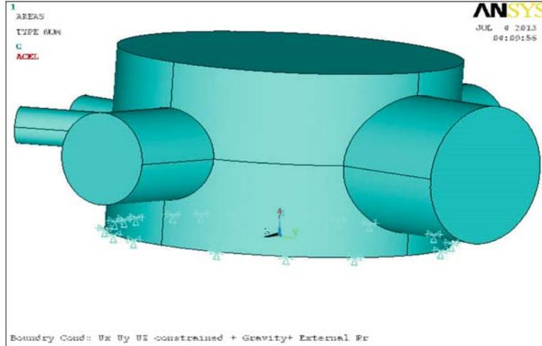
**Figure 2.** Typical load of the vacuum chamber.
