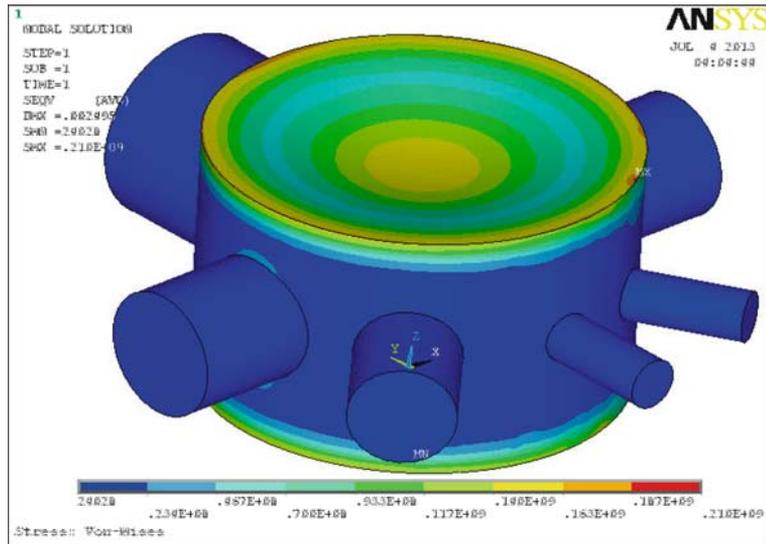
**Figure 3.** Von-Mises stress distribution (hot point stress at a very small area of 210 MPa and neglected due to elemental errors and rest zones are well below  $\sim 130$  MPa,  $<2/3$  of the yield strength of SS304L).
