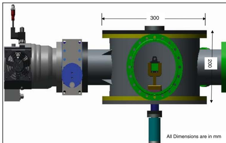
**Figure 4.** 3D view of the scattering chamber.
