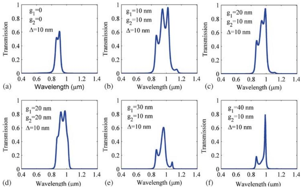
**Figure 6.** The transmission spectrum of the plasmonic filter containing two ring resonators with narrow gaps.
