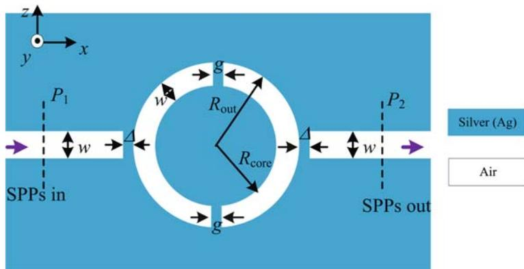
**Figure 1.** Schematic diagram of the MIM plasmonic filter with a circular ring resonator.  $w$ ,  $R_{\text{core}}$  and  $R_{\text{out}}$  are the width of the MIM waveguide, the radius of the core and the outer radius of the ring resonator, respectively.  $\Delta$  is the coupling length between the waveguide and the resonator,  $g$  is the width of the narrow gap.
