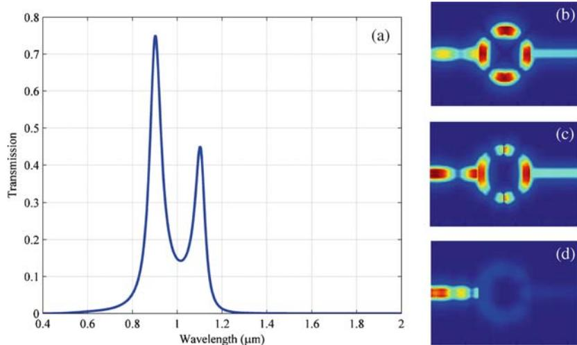
**Figure 3.** (a) The transmission spectrum of the MIM ring resonator with dual narrow gaps. The contour profiles of the field  $|H_y|^2$  of the nanoscale resonator at different wavelengths: (b)  $\lambda = 0.898 \mu\text{m}$ , (c)  $\lambda = 1.095 \mu\text{m}$  and (d)  $\lambda = 0.502 \mu\text{m}$ .
