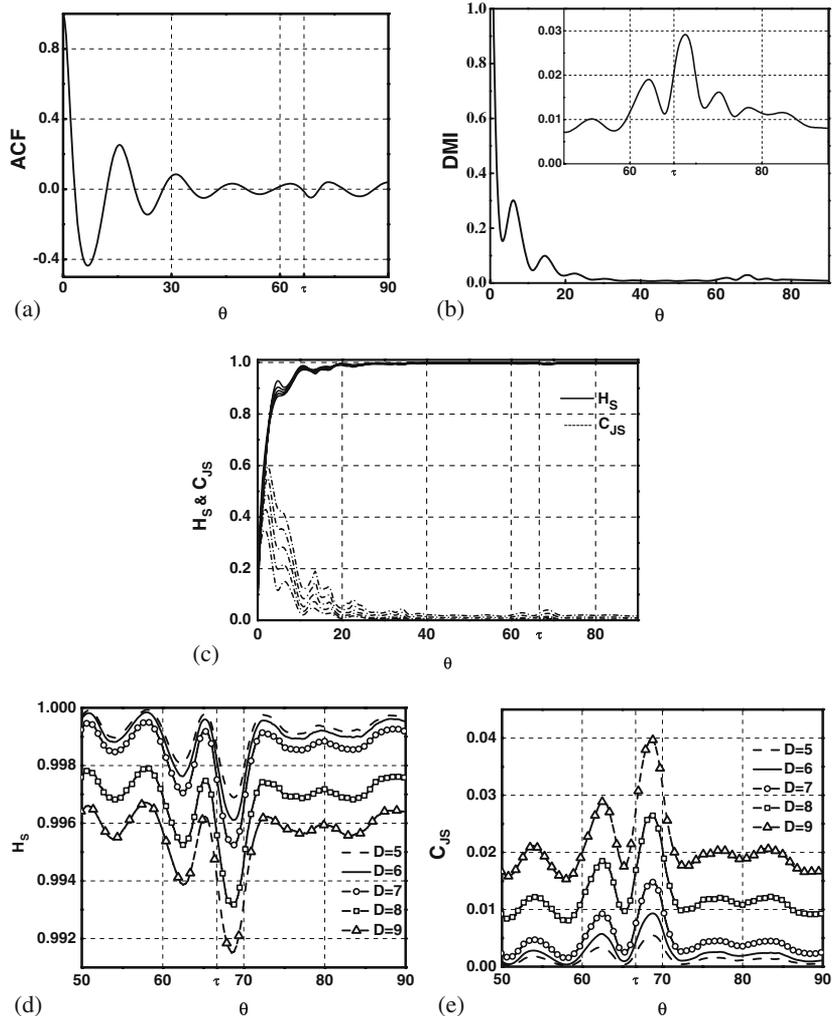
**Figure 1.** (a) ACF, (b) DMI, (c)  $H_S$  and  $C_{JS}$  calculated from the output intensity time series of QDL for  $\tau = 400$  ps and  $\gamma = 0.18$ . For  $H_S$  and  $C_{JS}$ ,  $D$  is varied from 5 to 9. (d) and (e) show enlarged parts of  $H_S$  and  $C_{JS}$  respectively, near the value of  $\tau$ .
