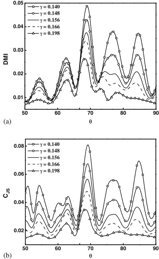
**Figure 4.** (a) DMI and (b)  $C_{JS}$  calculated for six different values of feedback rate ( $\gamma$ ) with  $\tau = 66.66$  (400 ps).
