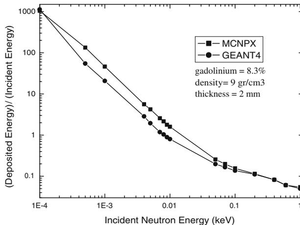
**Figure 5.** Total absorbed energy vs. incident neutron energy.
