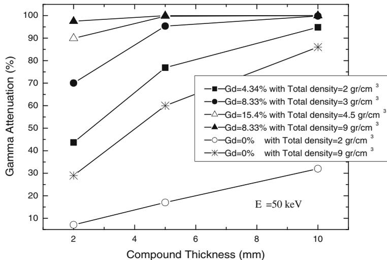
**Figure 1.** Attenuation of 50 keV  $\gamma$ -rays vs. thickness for different gadolinium atomic fractions and total compound densities.
