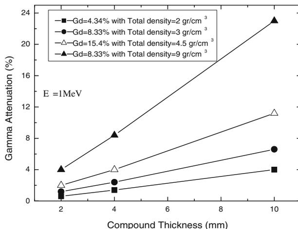
**Figure 3.** Attenuation of 1 MeV  $\gamma$ -rays vs. thickness for different gadolinium atomic fractions and total compound densities.
