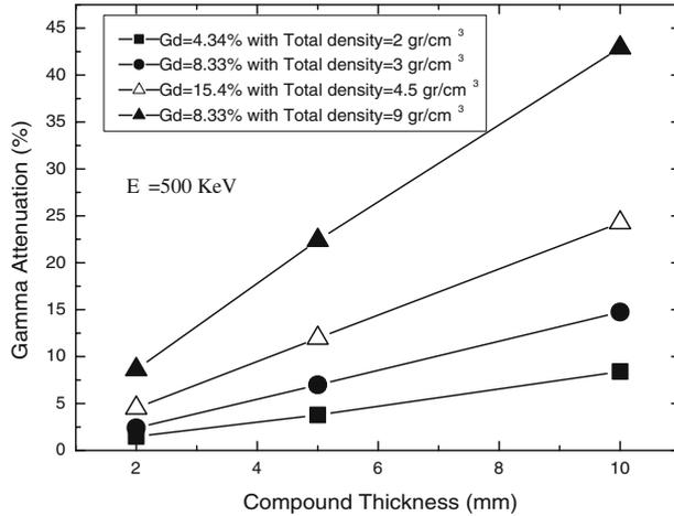
**Figure 2.** Attenuation of 500 keV  $\gamma$ -rays vs. thickness for different gadolinium atomic fractions and total compound densities.
