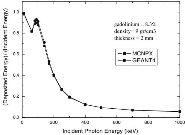
**Figure 4.** Total absorbed energy vs. incident gamma energy.
