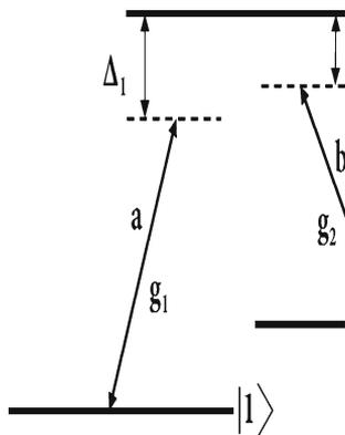
**Figure 1.** Three-level system with levels  $\{|0\rangle, |1\rangle, |2\rangle\}$  interacting with the cavity annihilation operators  $a$  and  $b$  with atom–cavity couplings  $g_1$  and  $g_2$  respectively. The respective one-photon detunings are  $\{\Delta_1, \Delta_2\}$ .
