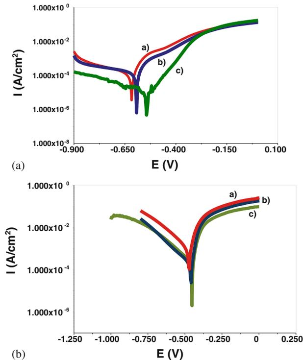
**Figure 5.** Potentiodynamic polarization curves of the bare SS (Curve a), TiO<sub>2</sub>/SS (Curve b) and PS/TiO<sub>2</sub>/SS (Curve c) in the (a) NaCl (1 M) and (b) H<sub>2</sub>SO<sub>4</sub> (1 M) solutions.
