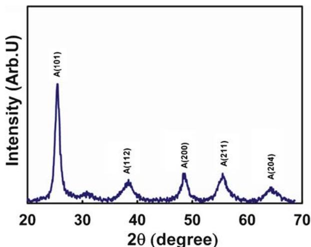
Figure 2. XRD pattern of the dip-coated  $\text{TiO}_2$  film.
