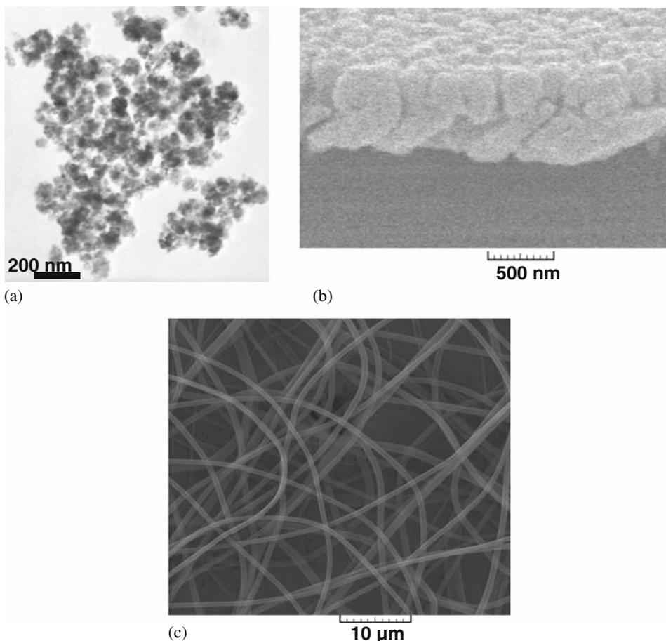
**Figure 1.** (a) TEM image of the scratched TiO<sub>2</sub> film, (b) SEM image of the cross-section of the TiO<sub>2</sub> film and (c) the PS fibres.
