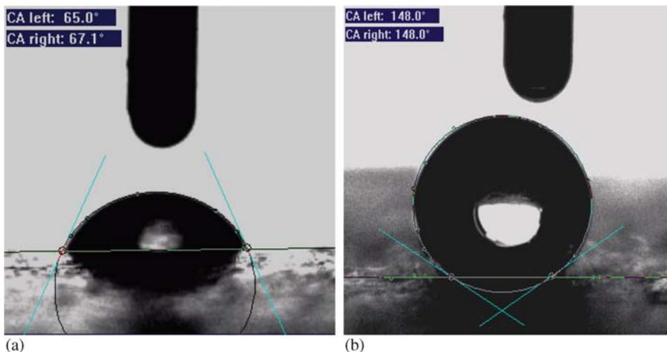
**Figure 3.** Results of contact angle measurements for (a) TiO<sub>2</sub>/SS and (b) PS/TiO<sub>2</sub>/SS samples.
