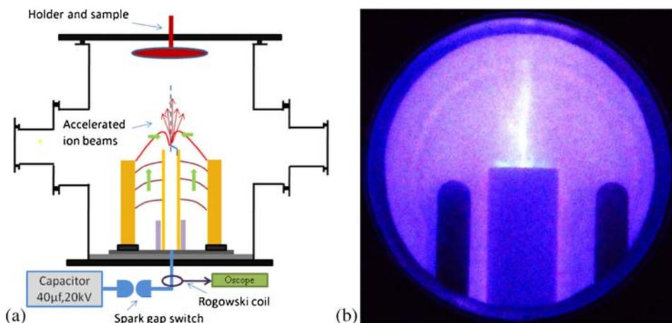
**Figure 2.** (a) A scheme of the APF plasma focus device as an ion beam accelerator and (b) a picture of the dense plasma column produced by the APF plasma focus device.
