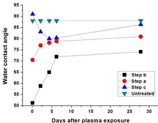
**Figure 5.** Water contact angle as a function of aging time after plasma treatment.
