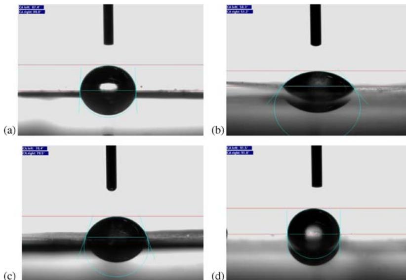
**Figure 4.** Visual comparison of the improvement in hydrophilicity: (a) before treatment, (b) for step (b), (c) for step (a) and (d) for step (c).
