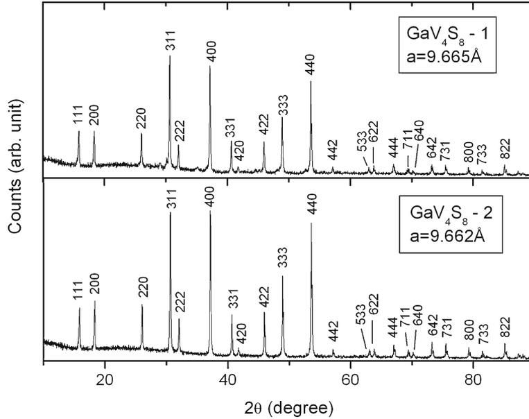
**Figure 1.** X-ray diffraction of GaV<sub>4</sub>S<sub>8</sub>-1 and GaV<sub>4</sub>S<sub>8</sub>-2 at room temperature.
