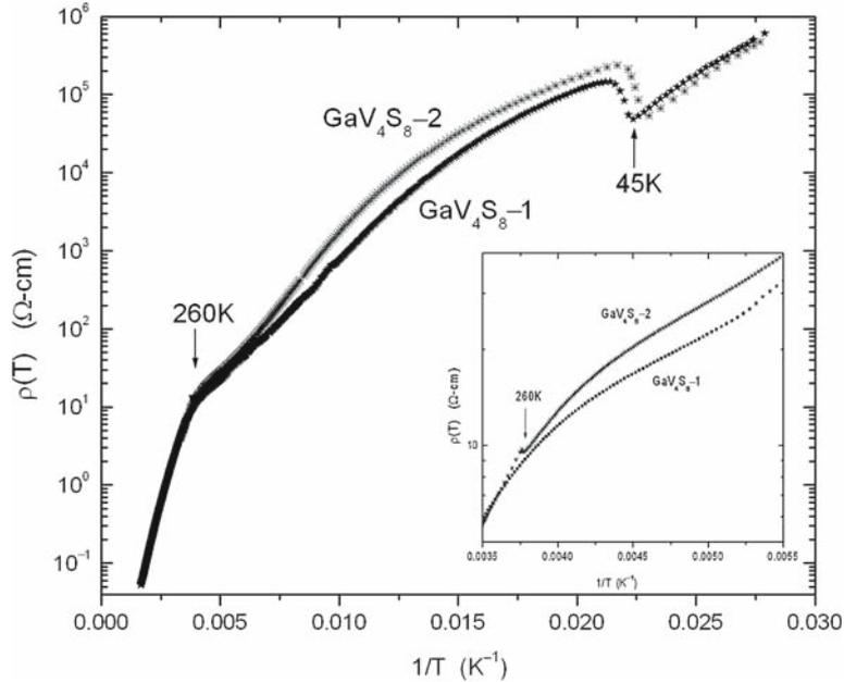
**Figure 2.** Log  $\rho$  vs.  $1/T$  plot for  $\text{GaV}_4\text{S}_8$ -1 annealed at  $800^\circ\text{C}$  and  $\text{GaV}_4\text{S}_8$ -2 annealed at  $500^\circ\text{C}$ . Inset figure shows the change in log  $\rho$  around 260 K in  $\text{GaV}_4\text{S}_8$ -1 and  $\text{GaV}_4\text{S}_8$ -2.
