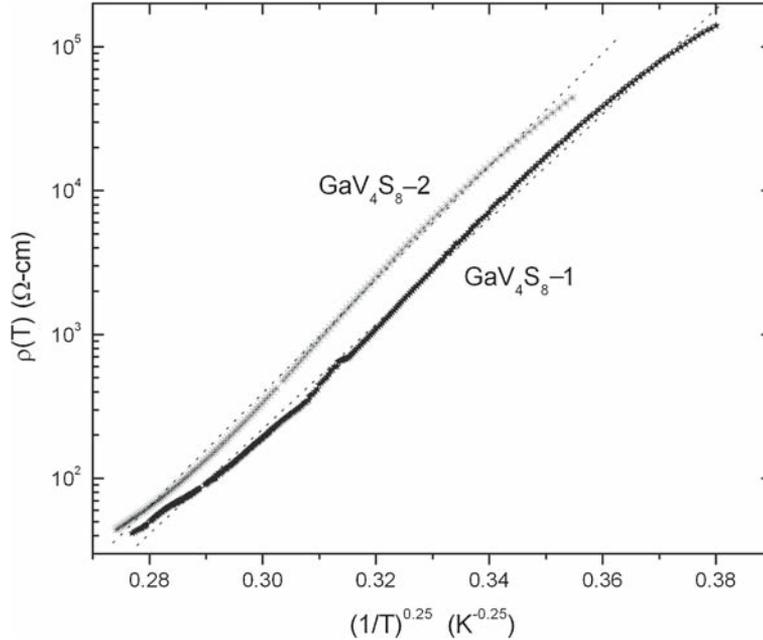
**Figure 3.** Mott's law,  $\log \rho$  vs.  $(1/T)^{1/4}$  well fitted in the non-Arrhenius region of  $\text{GaV}_4\text{S}_8-1$  and  $\text{GaV}_4\text{S}_8-2$ .
