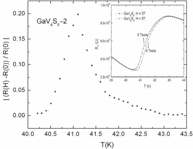
**Figure 4.** Magnitude of magnetoresistance vs. temperature below 43 K in  $\text{GaV}_4\text{S}_8$ -2. Inset figure shows the resistance in the magnetic field  $H = 0$  T and 6 T in  $\text{GaV}_4\text{S}_8$ -2.
