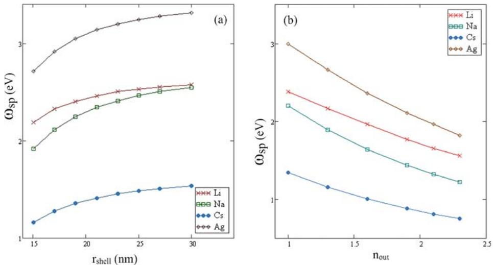
**Figure 6.** Surface plasmon energy as a function of (a) surrounding media having different refractive indices with  $r_{core} = 10$  nm,  $r_{shell} = 15$  nm,  $n_{core}(\text{SiO}_2) = 1.5$  and (b) outer radius shell with  $n_{out}(\text{H}_2\text{O}) = 1.3$ ,  $r_{core} = 10$  nm,  $n_{core}(\text{SiO}_2) = 1.5$ . Calculations presented are from different metallic nanoshell materials.
