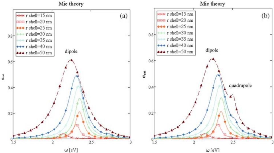
**Figure 4.** The extinction cross-section calculated based on the Mie theory for the nanoshell with a constant radius of the core and different radii of the shell, (a) for dipole mode SPR and (b) for both dipole and quadrupole SPR.
