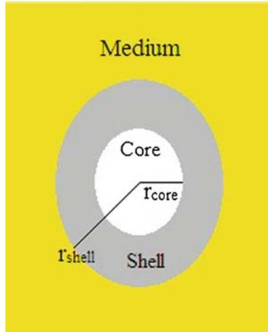
**Figure 1.** Schematic representation of the metal nanoshell with dielectric (core) and metal (nanoshell).
