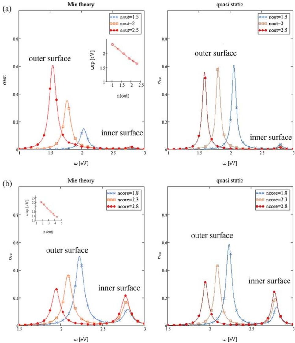
**Figure 3.** The extinction cross-section calculated for gold nanoshells using quasistatic approximation and Mie theory for (a) different embedding medium refractive index with  $n_{\text{core}}(\text{SiO}_2) = 1.5$  and (b) the different core with  $n_{\text{out}}(\text{H}_2\text{O}) = 1.3$ .  $r_{\text{core}} = 10$  nm and  $r_{\text{shell}} = 15$  nm.
