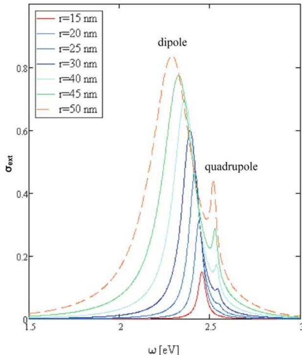
**Figure 5.** Extinction cross-section for gold nanospheres with radius ranging from 15 to 50 nm in a medium with  $n_{\text{out}} = 1.5$ .
