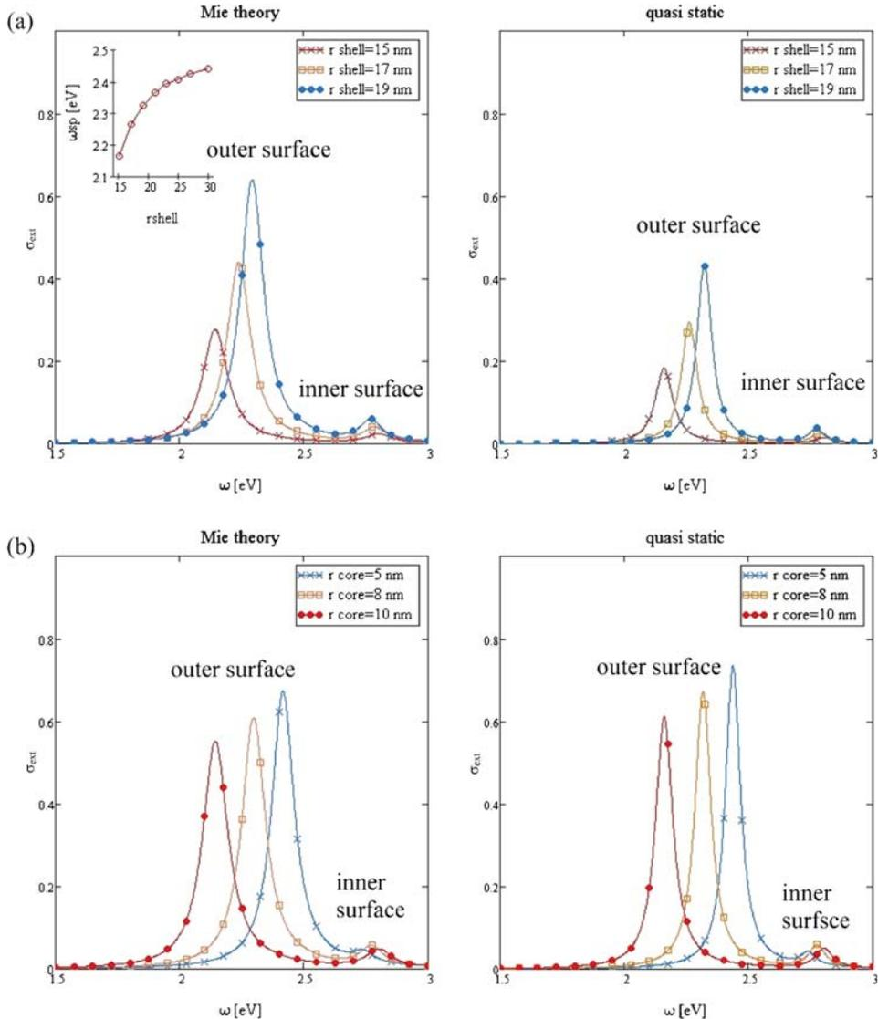
**Figure 2.** The extinction cross-section calculated for gold nanoshells using quasistatic approximation and Mie theory, (a) for core radius of 10 nm and different outer shell radii of 15, 17, 19 nm and (b) for a constant outer radius of 15 nm and different radii of the core embedded in a medium with  $n_{\text{out}} = 1.5$ . Inset shows the SPR response to a range of outer radii of the shell.
