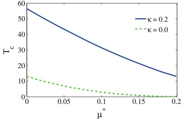
**Figure 2.** The transition temperature ( $T_c$ ) against Coulomb interaction coupling ( $\mu^*$ ) for the present theoretical system's optical phonon–electron interaction,  $\kappa = 0.2$  (blue, solid line) and for  $\kappa = 0.0$  (green, dashed line) for the parameters  $\lambda = 0.3$ ,  $\omega_a = 320$  K,  $\omega_p = 680$  K,  $\omega_c = 3$  eV.
