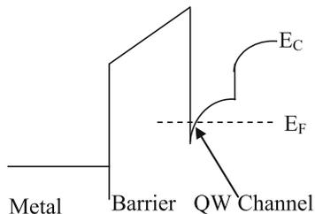
**Figure 3.** Quantum well/2DEG formation due to the conduction band discontinuity.
