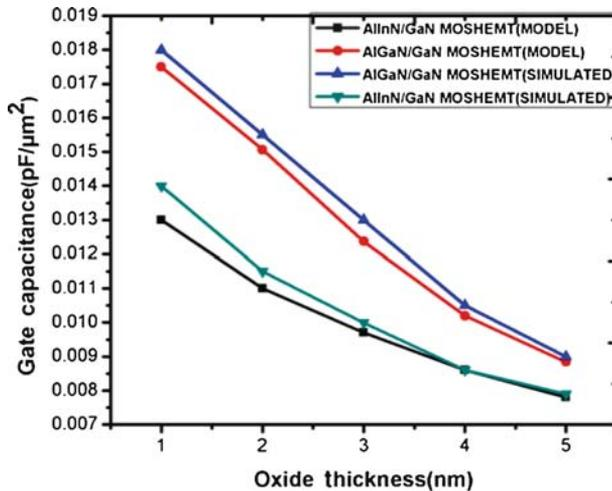
**Figure 7.** Plot showing gate capacitance ( $C_G$ ) vs. oxide thickness for AlInN/GaN and AlGaIn/GaN MOSHEMTs.
