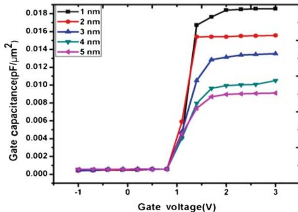
**Figure 9.** Plot showing gate capacitance vs. gate voltage for different oxide thicknesses in AlGaIn/GaN MOSHEMT.
