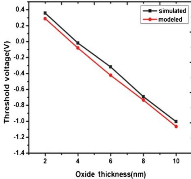
**Figure 6.** Plot showing threshold voltage ( $V_T$ ) vs. oxide thickness for AlInN/GaN MOSHEMT.
