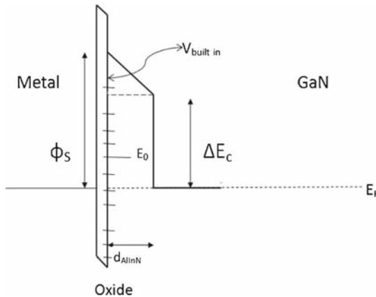
Figure 5. Conduction band at pinch-off.
