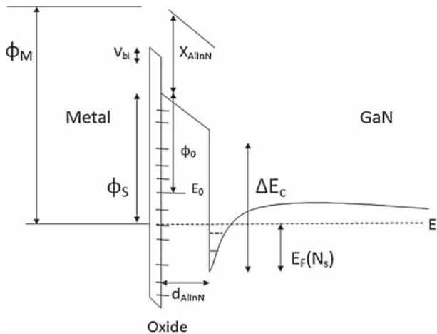
**Figure 4.** Conduction band profile for a metal/oxide/AlInN/GaN interface.
