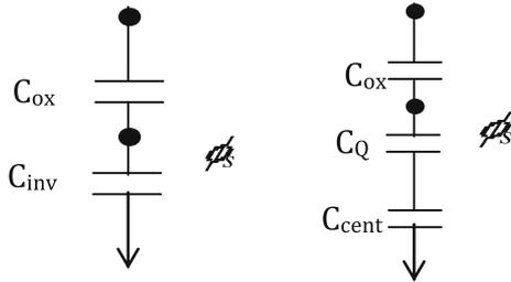
**Figure 2.** Equivalent circuit diagrams for gate capacitance in AlInN/GaN MOSHEMT.
