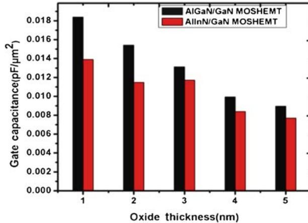
**Figure 10.** Plot showing gate capacitance vs. oxide thickness at a gate voltage of 2 V.
