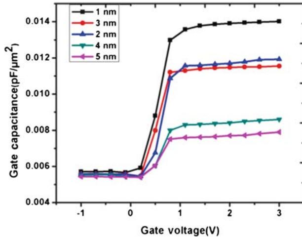
**Figure 8.** Plot showing gate capacitance vs. gate voltage for different oxide thicknesses of AlInN/GaN MOSHEMT.
