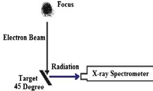
**Figure 4.** X-ray spectrometer position at the side-on of the system with the target at an angle of 45°.
