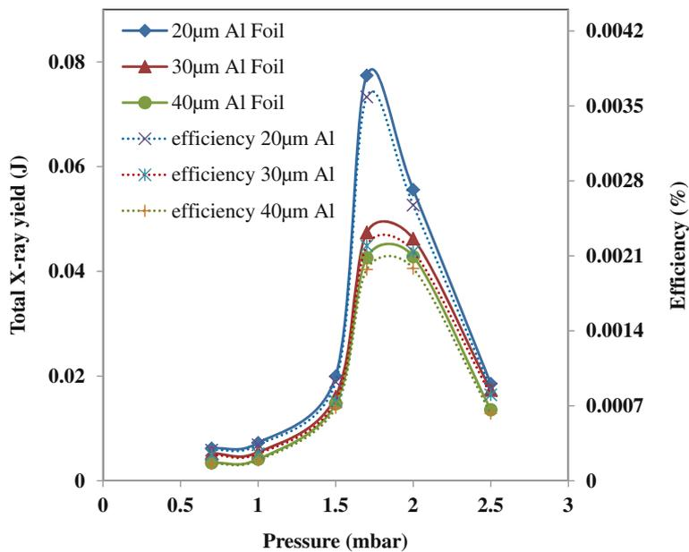
**Figure 9.** Variations of total X-ray yield in  $4\pi$ -geometry and efficiency vs. argon gas pressure at a constant applied voltage of 12 kV.
