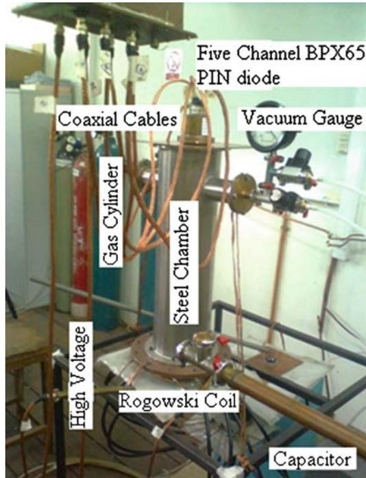
Figure 2. Picture of the plasma focus system.
