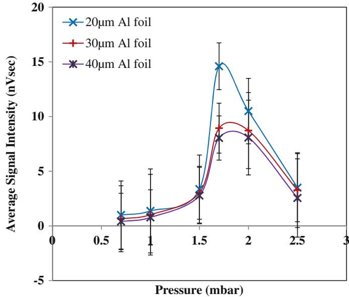
**Figure 8.** Variations in average signal intensities recorded at 20, 30, and 40  $\mu\text{m}$  Al foils vs. argon gas pressure.
