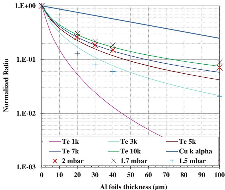
**Figure 10.** The calculated absorption curves of Al foils for X-rays from copper plasma at various temperatures and X-rays with argon gas pressures of 1.5, 1.7, and 2.0 mbar with the estimated electron temperatures 3, 7 and 6 keV, respectively.
