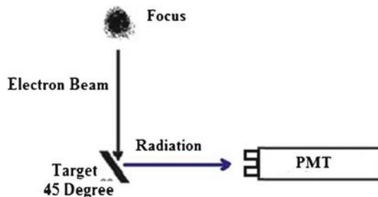
Figure 3. The R928 photomultiplier tube (PMT) coupled with a scintillator.
