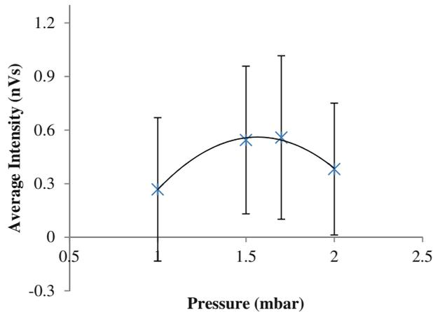
Figure 12. Variations of X-ray intensities with PMT vs. pressure (mbar).
