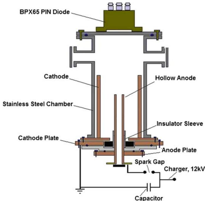
**Figure 1.** Schematic of the plasma focus device.
