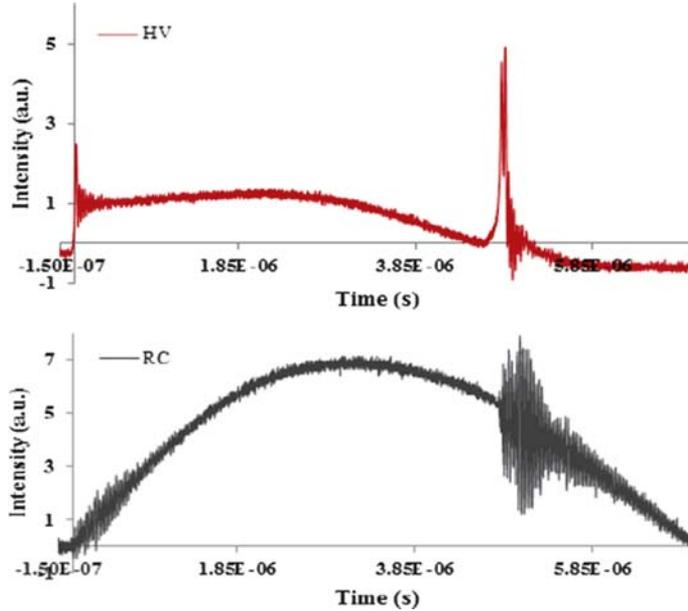
Figure 5. Typical Rogowski coil signal with high-voltage probe.
