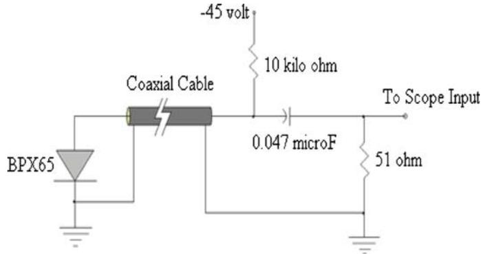
**Figure 6.** The basic circuit of the BPX65 PIN diode.
