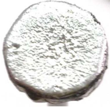
**Figure 14.** Picture of the lead target after bombardment of energetic electron beam from the focus.
