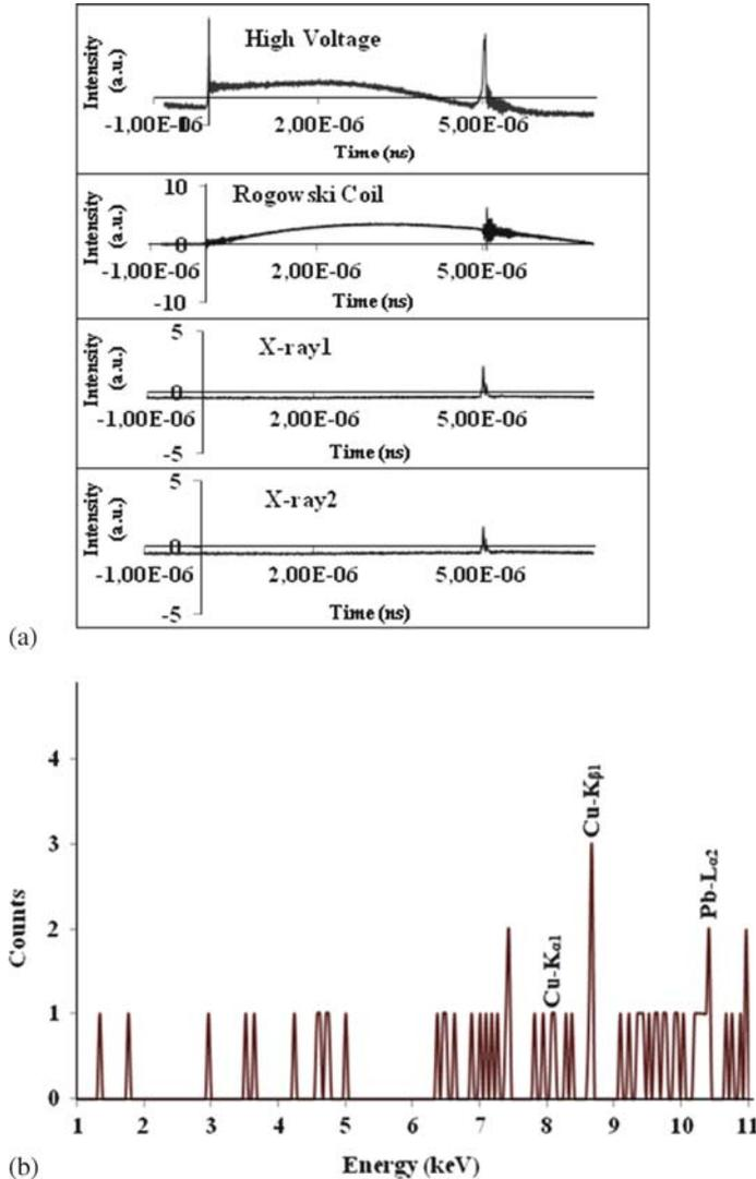
**Figure 13.** (a) Temporal evolution of X-ray pulses at a specific Al foil thickness for a pressure of 1.7 mbar, X-ray1 (23  $\mu\text{m}$  aluminized Mylar + 30  $\mu\text{m}$  Al foil), X-ray2 (23  $\mu\text{m}$  aluminized Mylar + 20  $\mu\text{m}$  Al foil) with the typical HV and RC signals. (b) X-ray spectrum: X-rays produced by the energetic electron beam target effect at an angle of 45° when the spectrometer is at side-on position.
