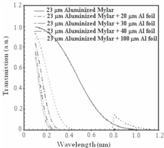
**Figure 7.** Transmission curves of 23  $\mu\text{m}$  aluminized Mylar, 23  $\mu\text{m}$  aluminized Mylar + (20, 30, 40, and 100  $\mu\text{m}$ ) Al foils.
